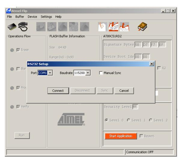
**Step 4**: Load hex file. On loading, the hex file name will be displayed in the center under flash buffer information along with size of it. Then, perform Erase, Blank Check, Program and Verify cycles.
