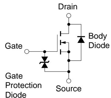
The diode connected between the gate and source of the transistor serves as a protector against ESD. When this device actually used, an additional protection circuit is externally required if a voltage exceeding the rated voltage may be applied to this device.
