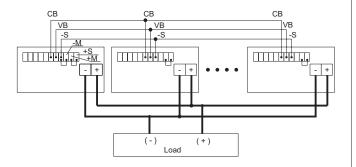
■In parallel operation, output voltage increases like stairs due to a delay of the rise time of output voltage at turn on.
