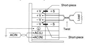
(2)When using remote sensing function
