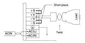
(2)When using remote sensing function
