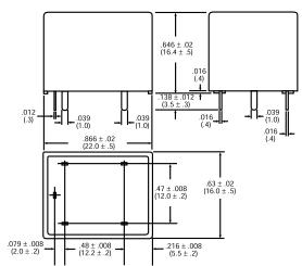
**Terminal assignment**Bottom view on solder pins
