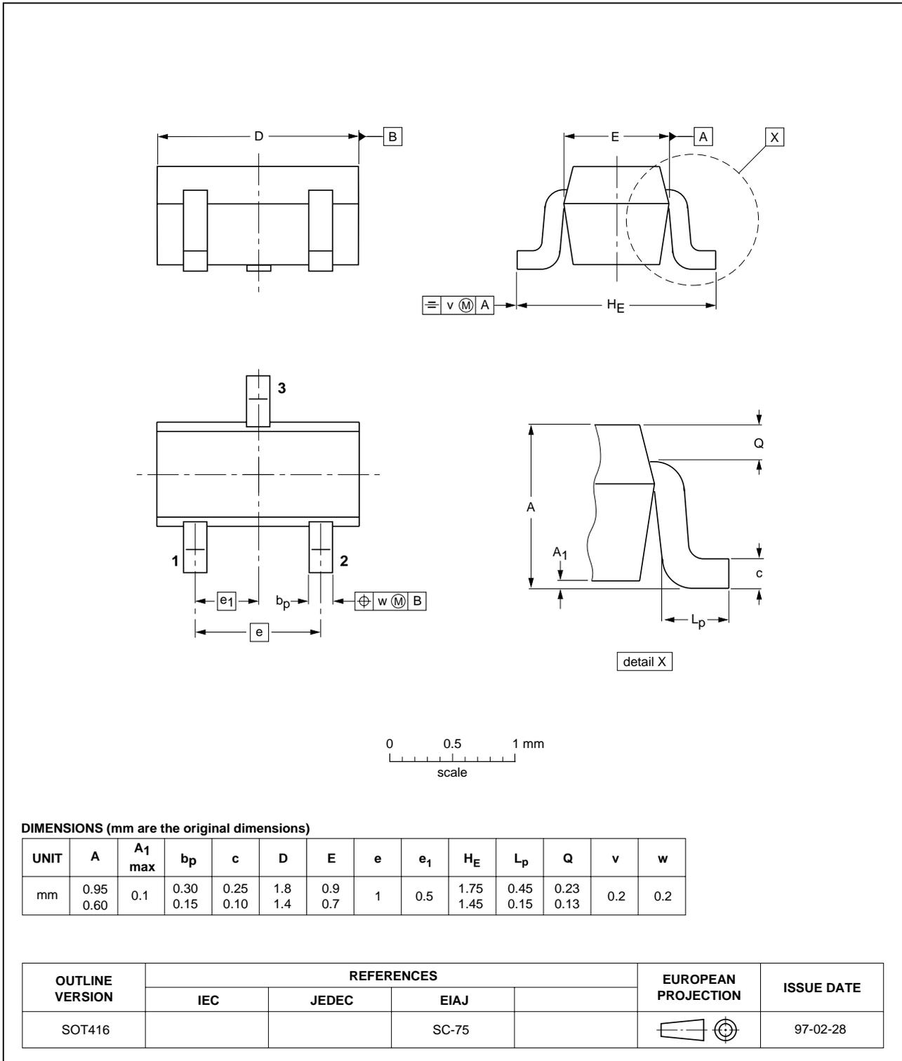
PNP resistor-equipped transistors;
