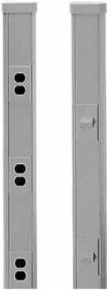
Cable ways provide a means for distributing power or data connections to each compartment in an isolated fashion. Non-metallic light-gray composite material. Both kits include cable runway with cover and two end caps with cable knockouts. Power Cable Way Kit also includes four dual category 5 RJ45 connectors and cover plates.
