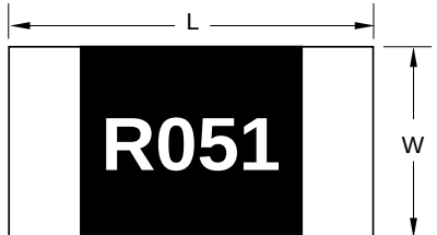
Fig. 5 Chip resistor outlines
