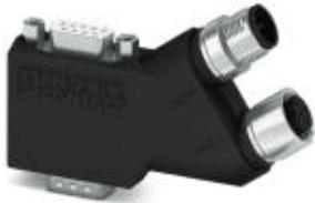
D-SUB plug, 9-pos., pin, with PG-D-SUB socket, assignment: 3, 5, 6, 8; two M12 cable glands (B-coded) under 35°. Bus system: PROFIBUS DP up to 12 Mbps. Termination resistor via separate M12 terminator.
