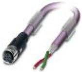
Bus system cable, PROFIBUS (12 Mbps), 2-position, PUR halogen-free, violet RAL 4001, shielded, free cable end, on Socket straight M12 SPEEDCON, B-coded, Cable length: Free input (0.2 ... 40.0 m)
