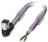
Bus system cable, PROFIBUS (12 Mbps), 2-position, PUR halogen-free, violet RAL 4001, shielded, free cable end, on Socket angled M12 SPEEDCON, B-coded, Cable length: Free input (0.2 ... 40.0 m)
