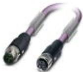
Bus system cable, PROFIBUS (12 Mbps), 2-position, PUR halogen-free, violet RAL 4001, shielded, Plug straight M12 SPEEDCON, B-coded, on Socket straight M12 SPEEDCON, B-coded, Cable length: 1 m
