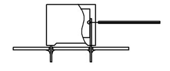
Temperature monitored inside the capacitor.
