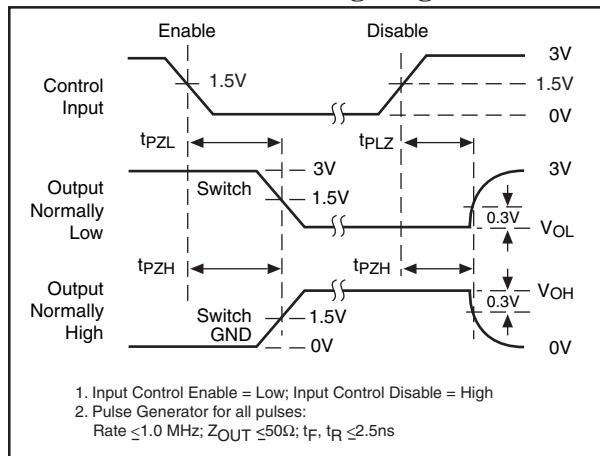
**Propagation Delay Diagram**
