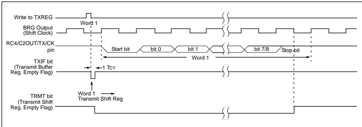
**FIGURE 18-4: ASYNCHRONOUS TRANSMISSION (BACK-TO-BACK)**
