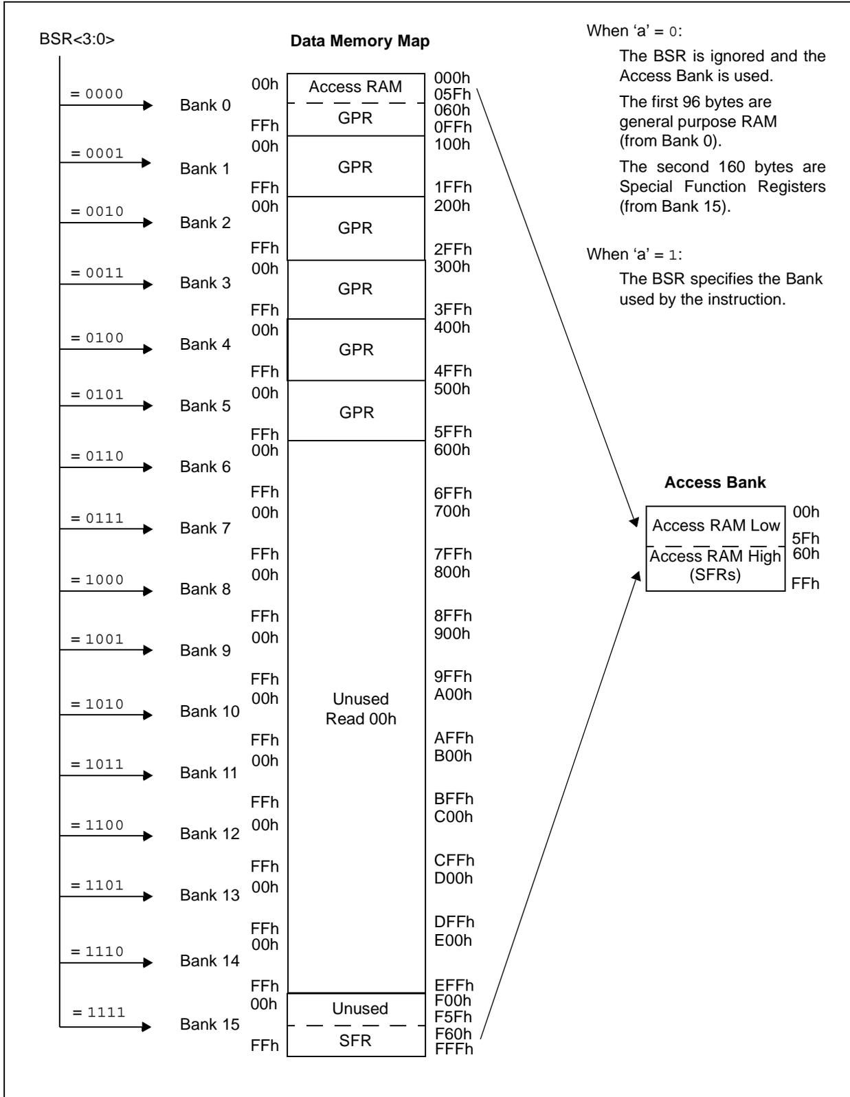
**FIGURE 5-8: DATA MEMORY MAP FOR PIC18F26K20/46K20 DEVICES**
