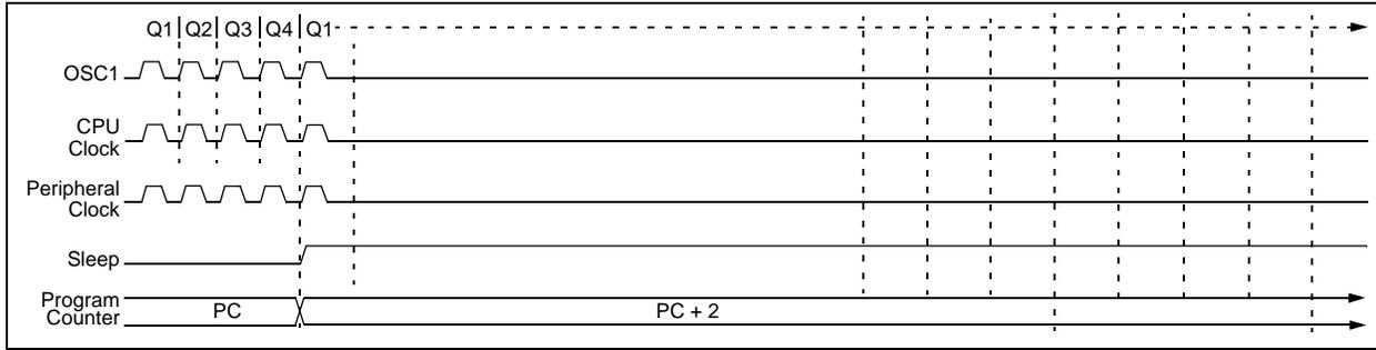
**FIGURE 3-2: TRANSITION TIMING FOR WAKE FROM SLEEP (HSPLL)**
