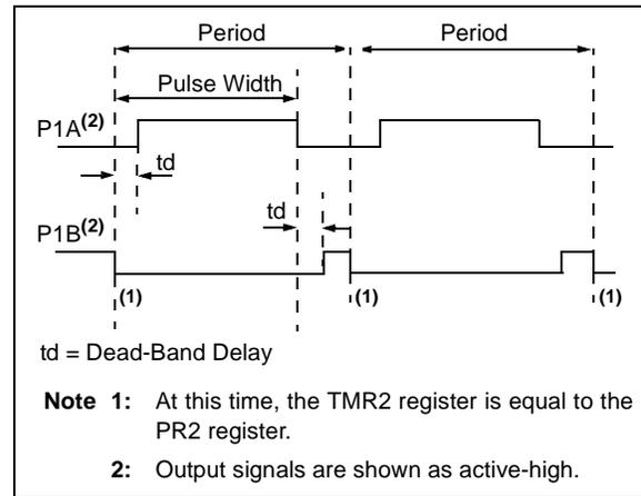
**FIGURE 16-5: EXAMPLE OF HALF-BRIDGE APPLICATIONS**
