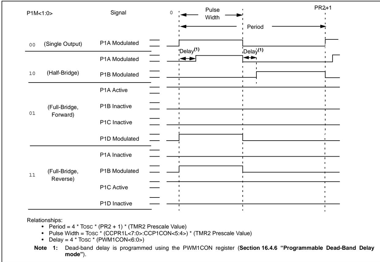
**FIGURE 16-3: EXAMPLE ENHANCED PWM OUTPUT RELATIONSHIPS (ACTIVE-LOW STATE)**
