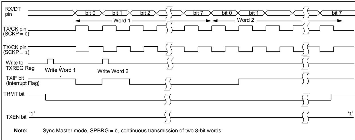
**FIGURE 18-11: SYNCHRONOUS TRANSMISSION (THROUGH TXEN)**
