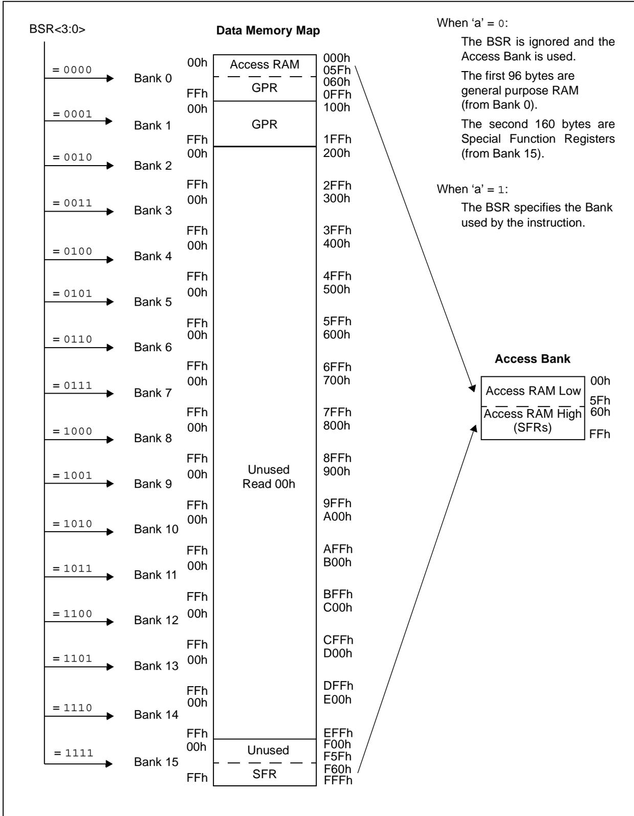
**FIGURE 5-6: DATA MEMORY MAP FOR PIC18F24K20/44K20 DEVICES**
