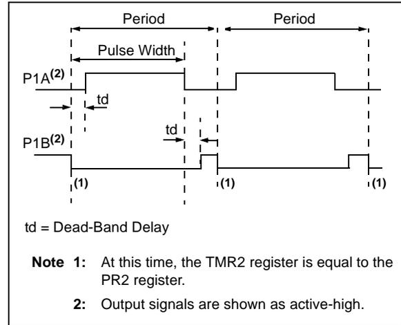
**FIGURE 16-13: EXAMPLE OF HALF-BRIDGE APPLICATIONS**
