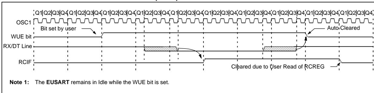
**FIGURE 18-8: AUTO-WAKE-UP BIT (WUE) TIMINGS DURING SLEEP**
