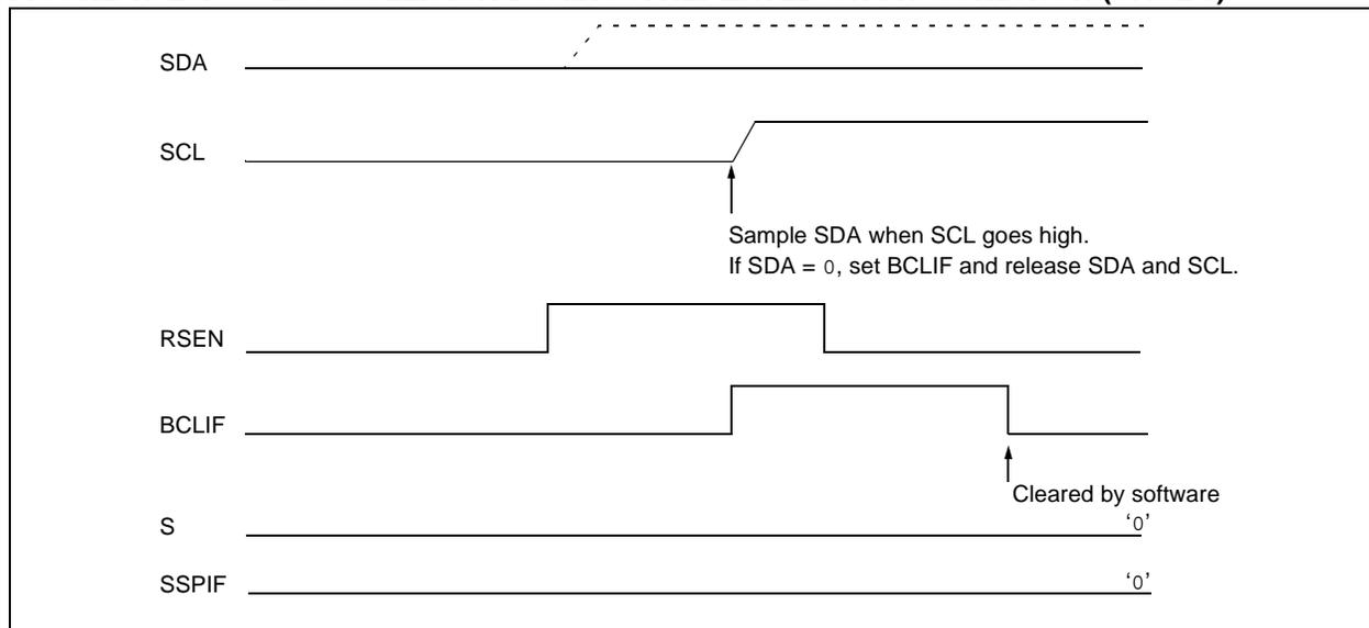
**FIGURE 17-30: BUS COLLISION DURING REPEATED START CONDITION (CASE 2)**
