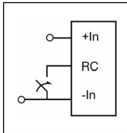
The products are fitted with a remote control function referenced to the primary negative input connection (- In), with negative and positive logic options available. The RC function allows the converter to be turned on/off by an external device like a semiconductor or mechanical switch. The RC pin has an internal pull up resistor to + In.
