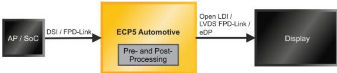
ECP5 can be used in a variety of other infotainment use cases as well, including splitting a single video output for dual rear-seat displays, and cropping and formatting video for a specific video resolution.
