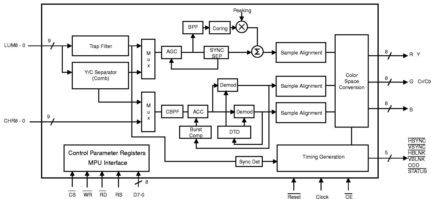
processed (odd or even). The detected synchronization signals are further processed and used for generating the synchronization signals for output from the decoder. (See the discussion for Data Output.)
