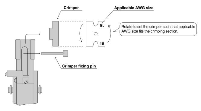
[Manual crimping tool: crimped section]
