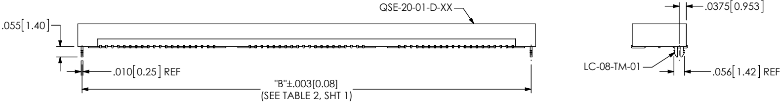
FIG 2 -LC: LOCKING CLIP OPTION (QSE-060-01-XXX-D-LC SHOWN) (DIFFERENT AS SHOWN, OTHERWISE SAME AS FIG 1)
