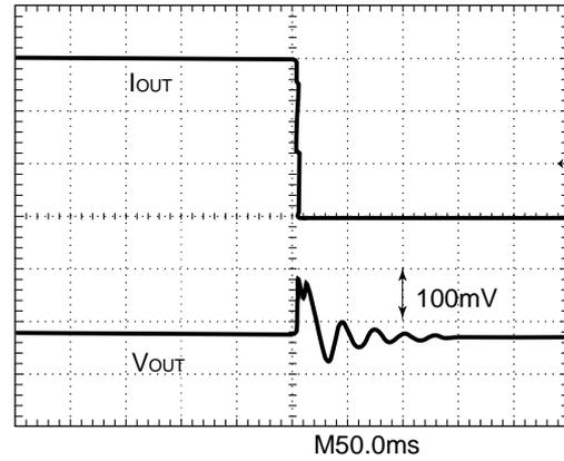
((R1210N302D)) ( $V_{IN}: 1.5V, I_{OUT}: 1mA \rightarrow 100mA$ )
