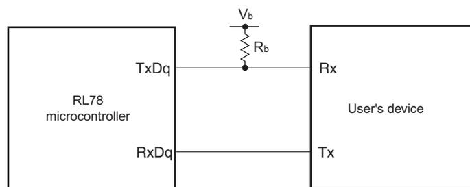
**UART mode bit width (during communication at different potential) (reference)**
