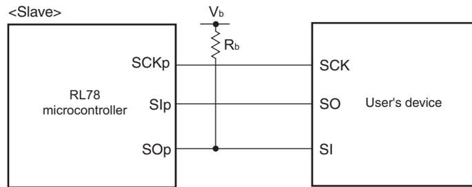
**CSI mode serial transfer timing (slave mode) (during communication at different potential)
