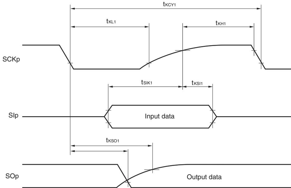
**CSI mode serial transfer timing (master mode) (during communication at different potential)**
