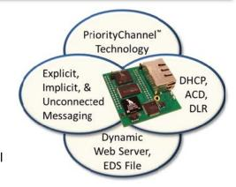
EtherNet/IP support includes Dynamic Host Configuration Protocol (DHCP) and Address Conflict Detection (ACD). Together, these two
