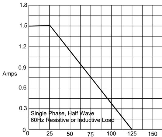
Average Forward Rectified Current - Amperes versus
