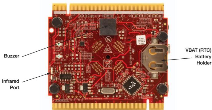
Figure 2: Back side of TWR-K20D50M module.
