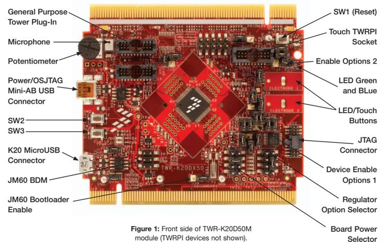
Figure 1: Front side of TWR-K20D50M module (TWRPI devices not shown).
