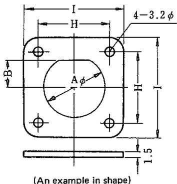
Square Flange is used with Bayonet Lock type receptacle.
