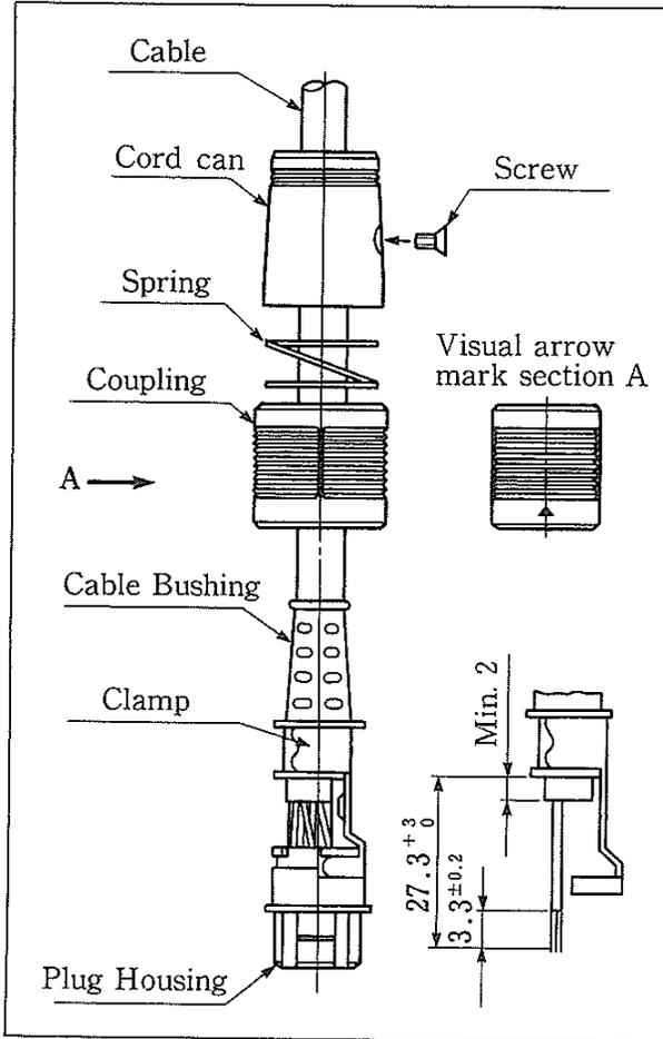
1. Fit the body, spring, coupling and bushing respectively in advance on wires having ends suitably treated, and then connect wires to terminals by crimp.
