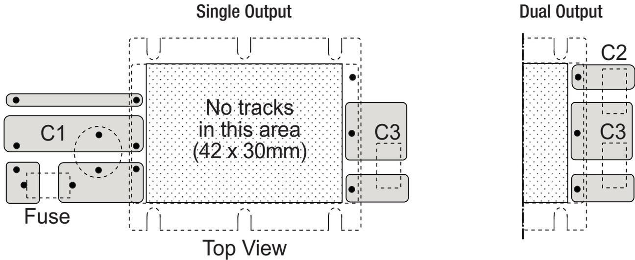
Input Fuse is recommended. Recommended fuse rating = double maximum input current, time delay type.
