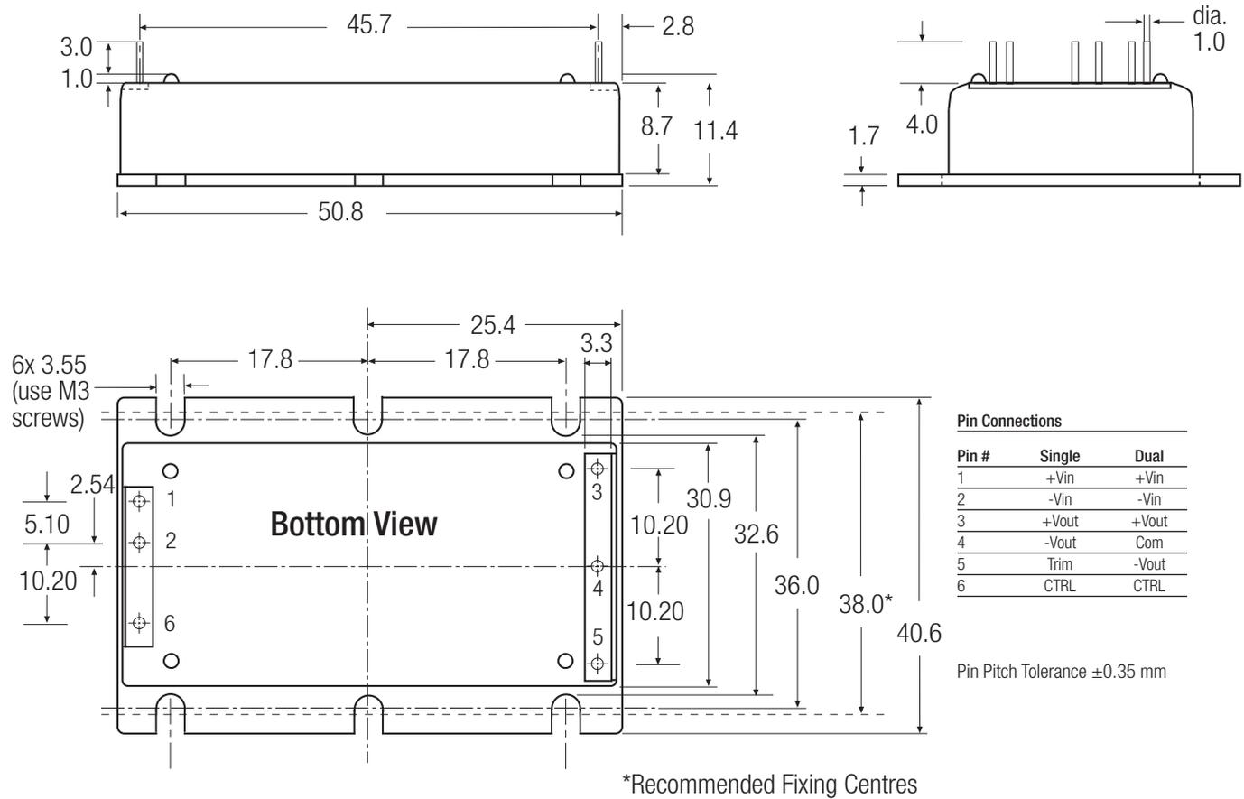
Baseplate Case Fixing - Mounting onto Heatsink/Bulkhead
