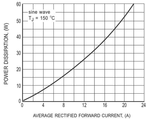
**FIG.2 POWER DISSIPATION**
