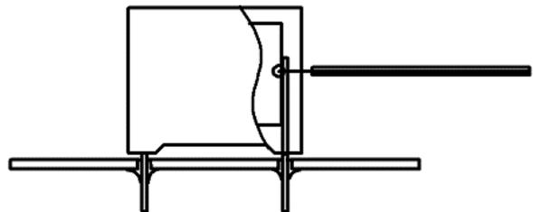
*Temperature monitored inside the capacitor.*
