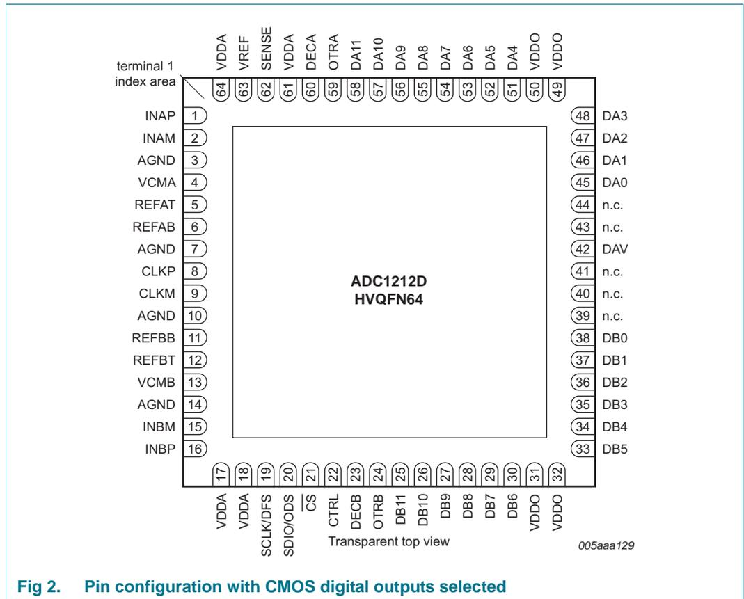
Fig 2. Pin configuration with CMOS digital outputs selected
