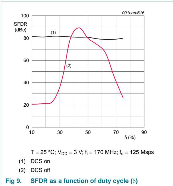
Fig 9. SFDR as a function of duty cycle ( $\delta$ )
