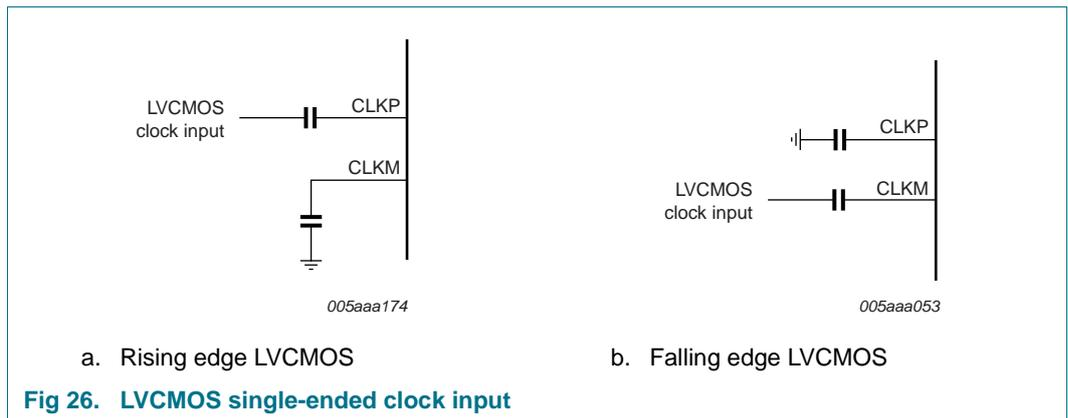
Fig 26. LVCMOS single-ended clock input
