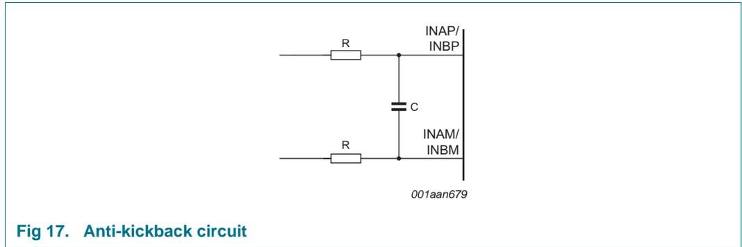
Fig 17. Anti-kickback circuit
