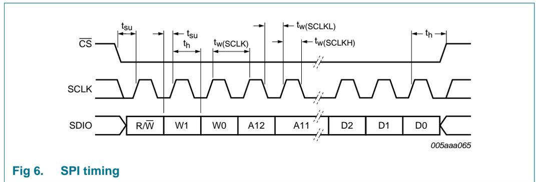
Fig 6. SPI timing
