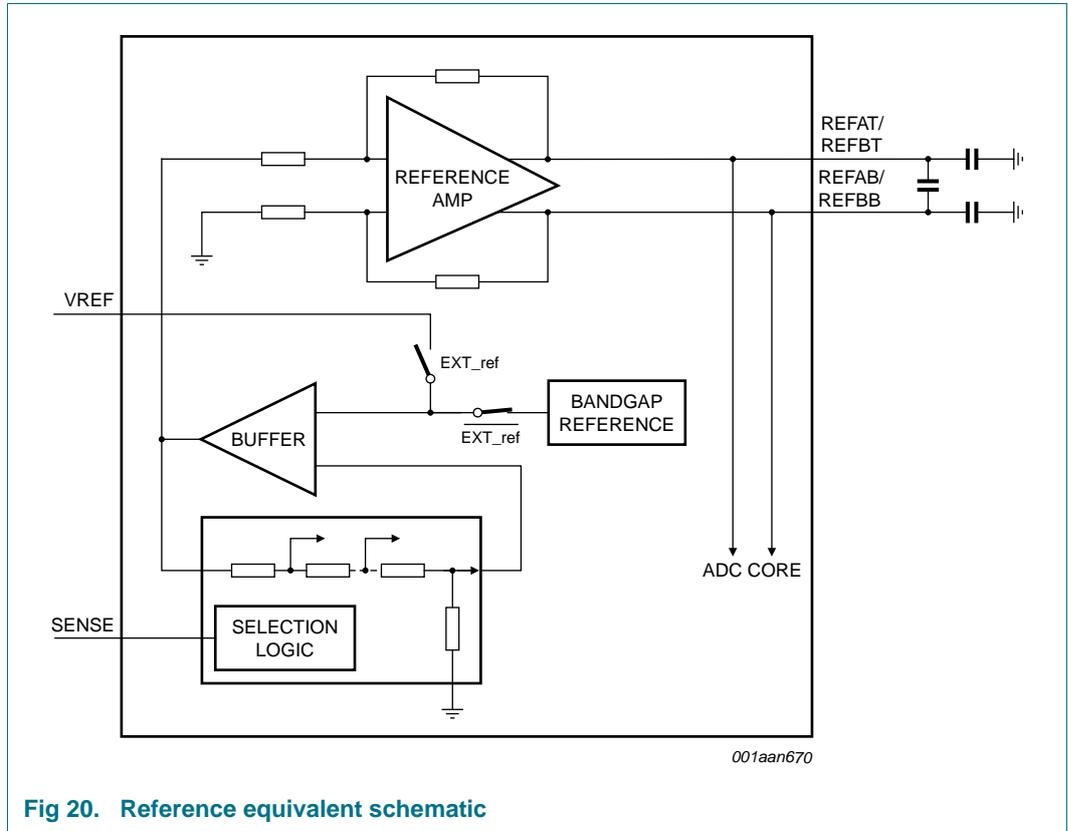
Fig 20. Reference equivalent schematic
