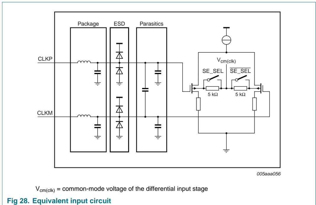
Single-ended or differential clock inputs can be selected via the SPI interface (see [Table 22](#)). If single-ended is enabled, the input pin (CLKM or CLKP) is selected via control bit SE\_SEL.
