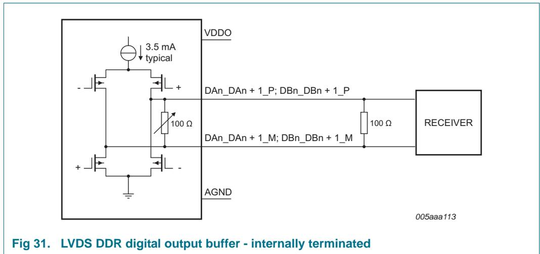
**Fig 31. LVDS DDR digital output buffer - internally terminated**
