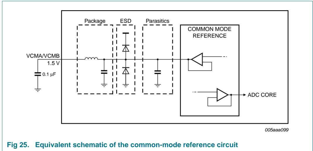
Fig 25. Equivalent schematic of the common-mode reference circuit
