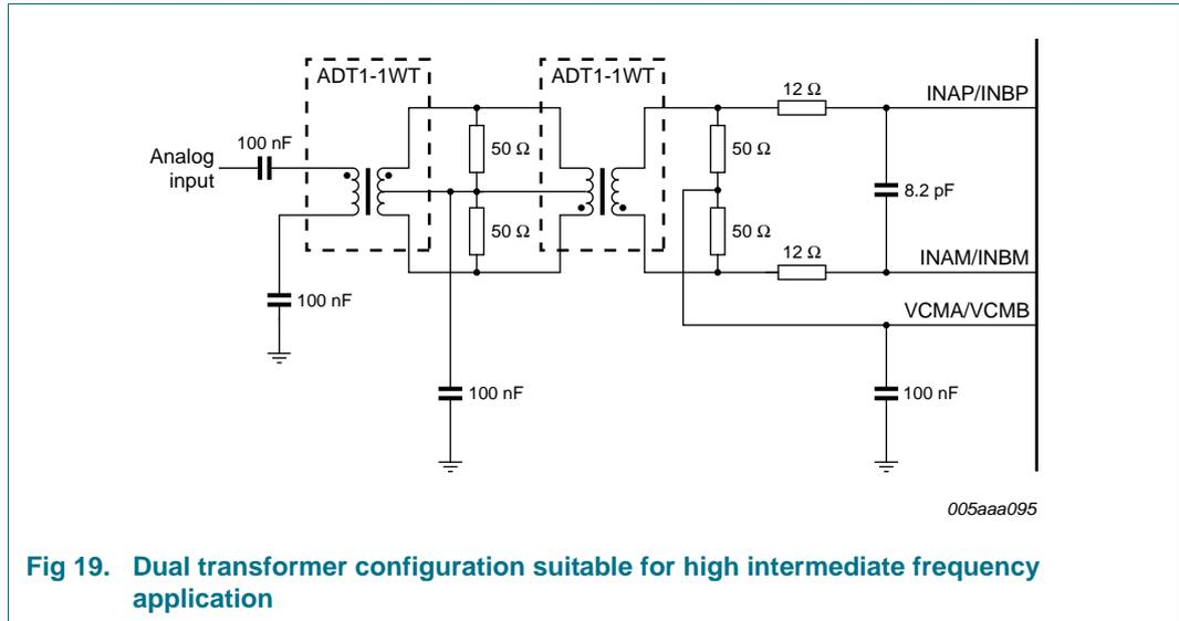
Fig 19. Dual transformer configuration suitable for high intermediate frequency application
