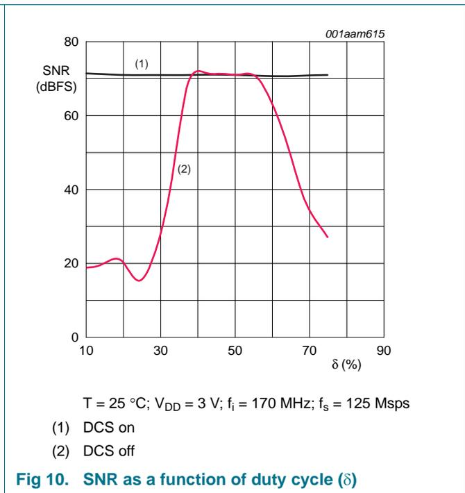
Fig 10. SNR as a function of duty cycle ( $\delta$ )
