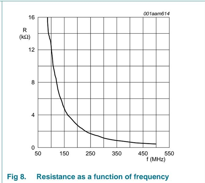
Fig 8. Resistance as a function of frequency
