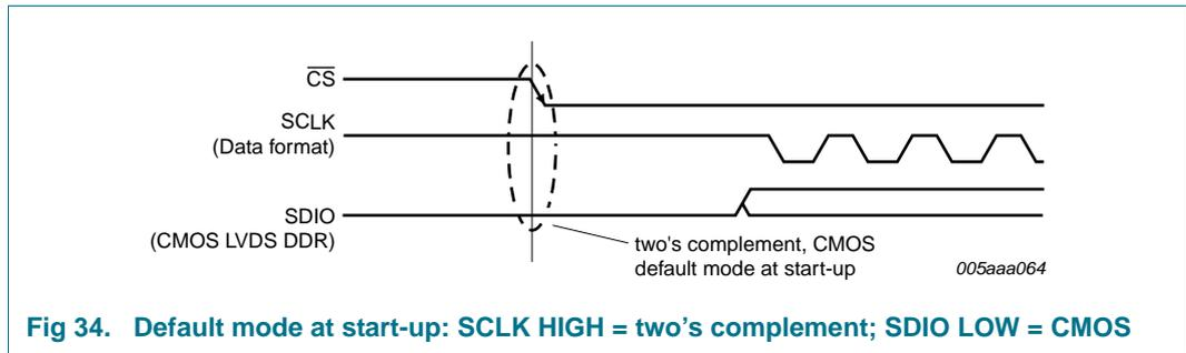
**Fig 34. Default mode at start-up: SCLK HIGH = two's complement; SDIO LOW = CMOS**
