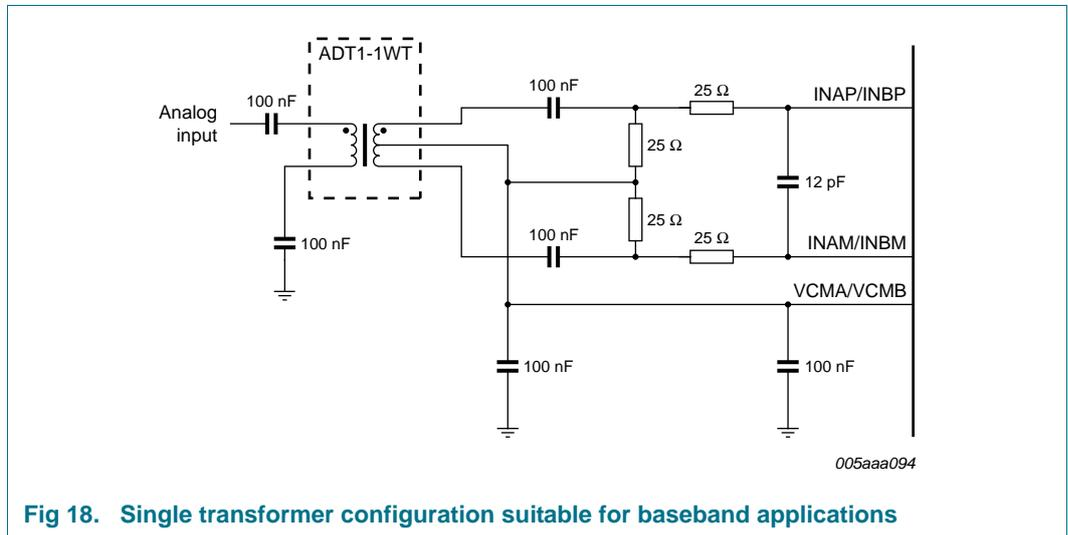
Fig 18. Single transformer configuration suitable for baseband applications
