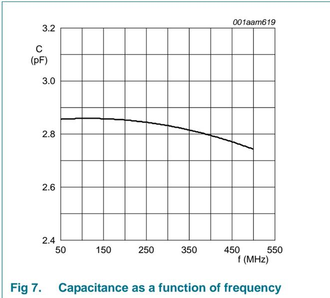
Fig 7. Capacitance as a function of frequency
