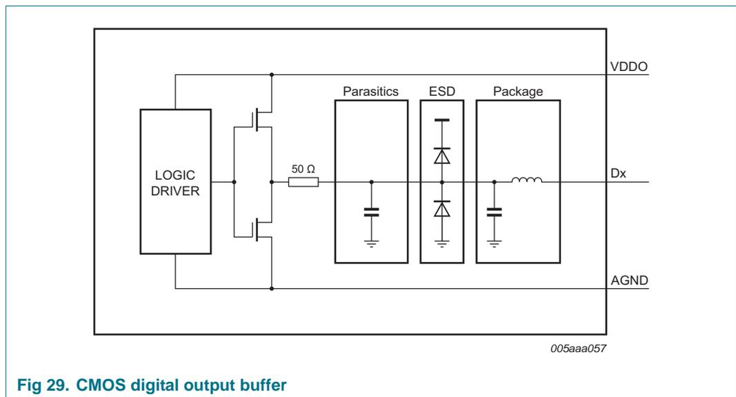
The output resistance is 50 Ω and is the combination of an internal resistor and the equivalent output resistance of the buffer. There is no need for an external damping resistor. The drive strength of both DATA and DAV buffers can be programmed via the SPI in order to adjust the rise and fall times of the output digital signals (see [Table 31](#)).
