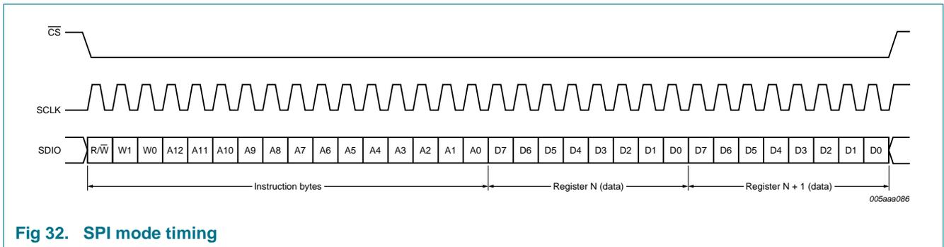
Fig 32. SPI mode timing
