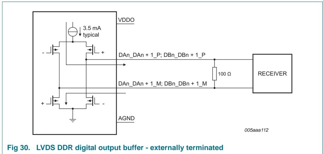
**Fig 30. LVDS DDR digital output buffer - externally terminated**
