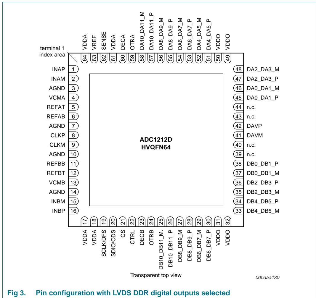
Fig 3. Pin configuration with LVDS DDR digital outputs selected
