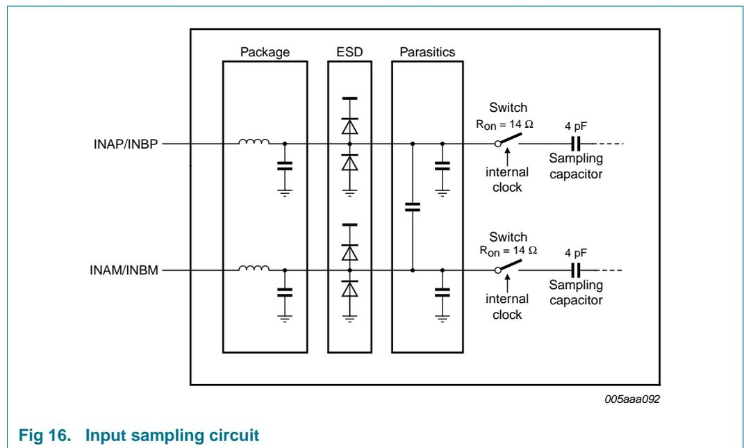
Fig 16. Input sampling circuit
