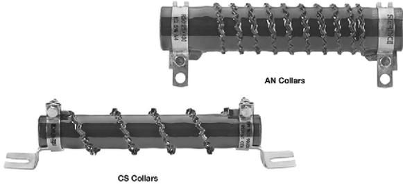
The remarkable dissipation power of this series is the result of an original winding method using corrugated edge-wound tape, thus forming a very active radiator. The enamelling follows the contour of the resistive element and provides effective insulation and support for the winding.
