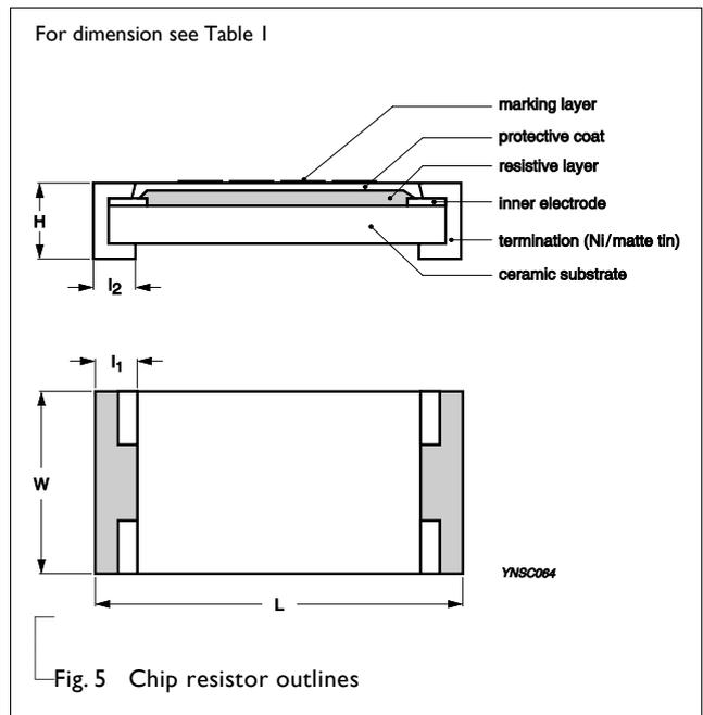
Fig. 5 Chip resistor outlines
