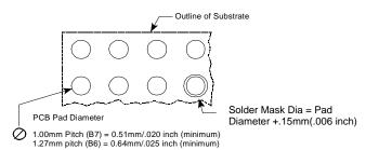
For .006" Thick Solder Paste Stencil, Aperture Opening Should be Equal to the PCB Pad Diameter.
