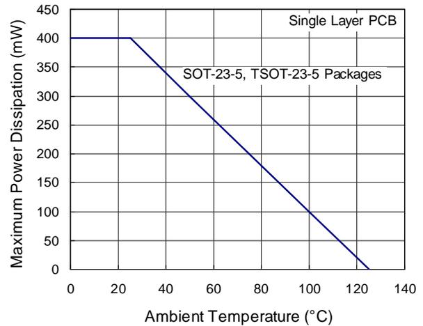
Figure 5. Derating Curves for RT8009 Package
