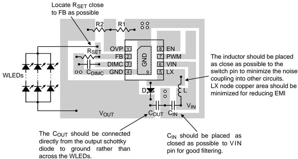
Figure 7. PCB Layout Guide
