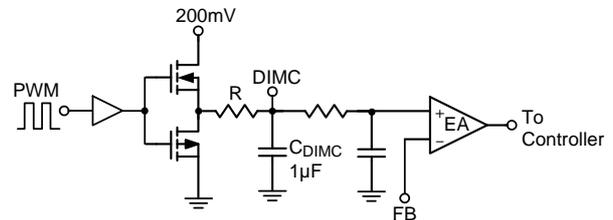
Figure 3. Block Diagram of Programmable FB Voltage.
