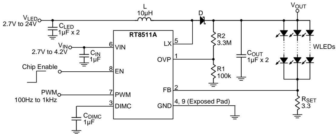
Figure 2. Typical Application Circuit of Low Voltage Operation
