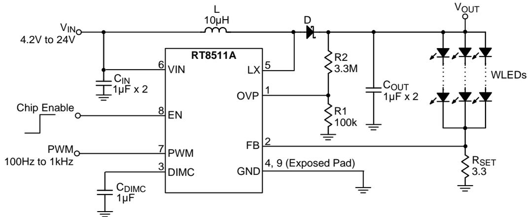
Figure 1. Typical Application Circuit of Normal Operation
