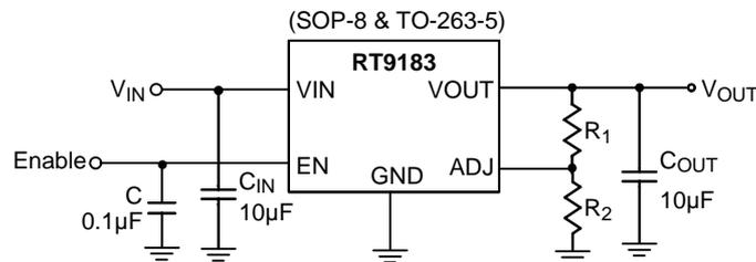
$$V_{OUT} = 0.8 \times \left(1 + \frac{R1}{R2}\right) \text{Volts}$$
