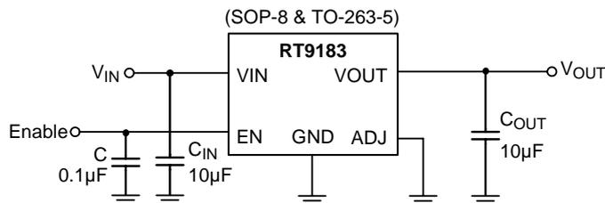
Figure 3. Fixed Operation with SOP-8 and TO-263-5 packages
