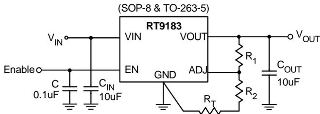
Figure 5. Return Pin of External Resistor Connection
