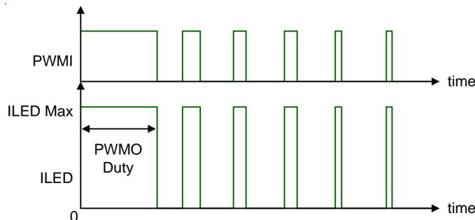
Figure 1. PWM Dimming
