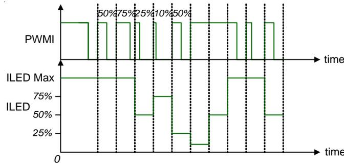
Figure 2. DC Dimming
