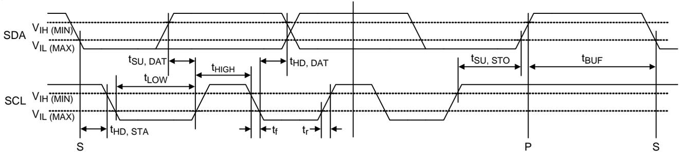
RT8555 I<sup>2</sup>C slave address = 7'b0110\_001. I<sup>2</sup>C interface support fast mode (bit rate up to 400kb/s). The write or read bit stream ( $N \geq 1$ ) is shown below
