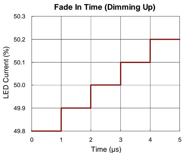
Figure 6. LED Current (Dimming Up) vs. Fade IN Time
