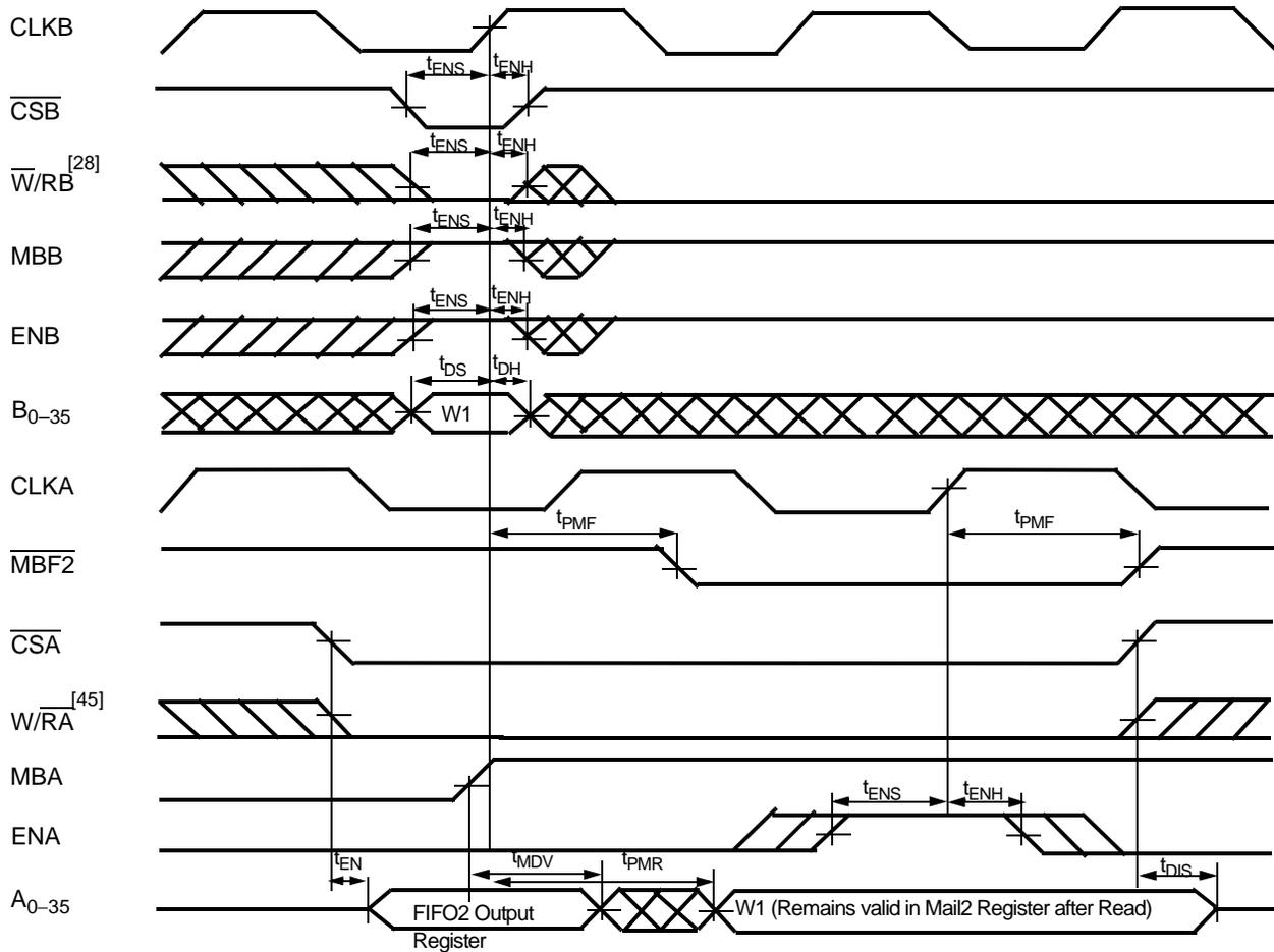
**FIFO Retransmit Timing<sup>[46, 47, 48, 49, 50]</sup>**
