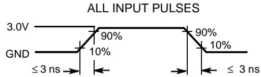
**AC Test Loads and Waveforms (-7)**
