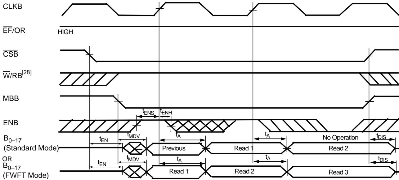
**Port B Byte Read Cycle Timing for FIFO (CY Standard and FWFT Modes)<sup>[30]</sup>**
