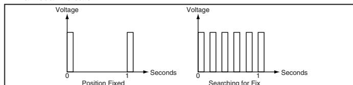
Figure 3: SG Series Lock Indicator Signals
