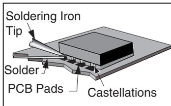
Figure 10: Soldering Technique
