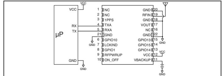
Figure 4: SG Series Module with a Passive Antenna
