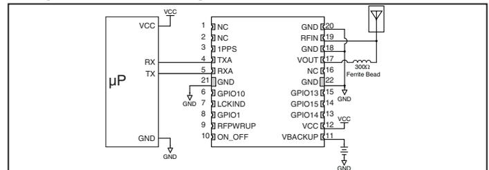
Figure 5: SG Series Module with an Active Antenna
