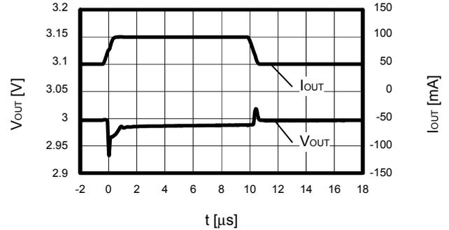
**(3) ON/OFF pin transient response characteristics**
