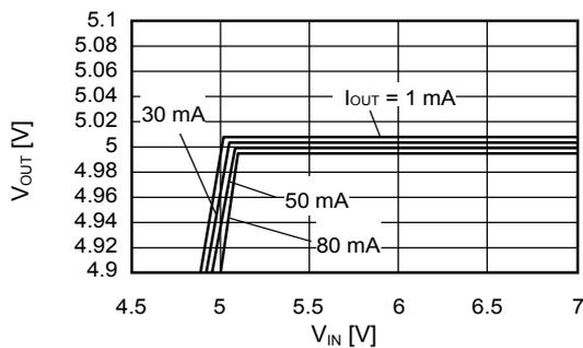
**(3) Dropout voltage vs. Output current**
