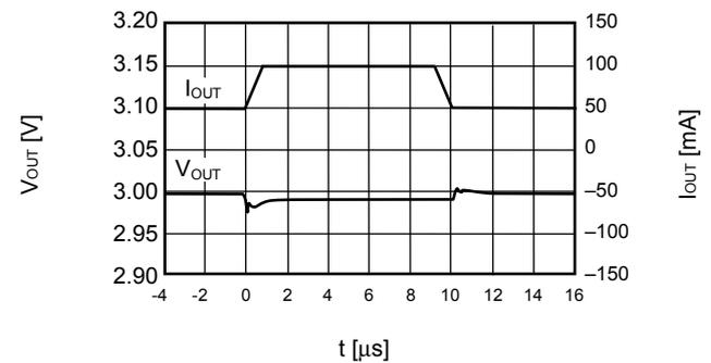
$V_{IN} = 4.0\text{ V}$ ,  $C_{OUT} = 2.2\ \mu\text{F}$ ,  $C_{IN} = 1.0\ \mu\text{F}$ ,  $I_{OUT} = 50\text{ mA} \leftrightarrow 100\text{ mA}$
