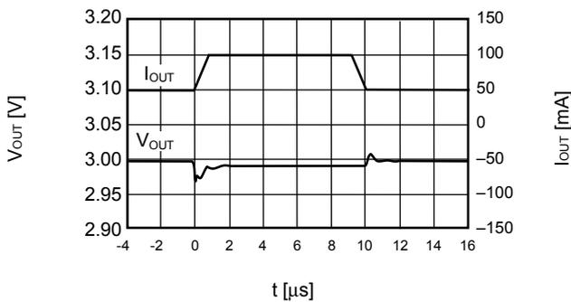
$V_{IN} = 4.0\text{ V}$ ,  $C_{OUT} = 1.0\ \mu\text{F}$ ,  $C_{IN} = 1.0\ \mu\text{F}$ ,  $I_{OUT} = 50\text{ mA} \leftrightarrow 100\text{ mA}$
