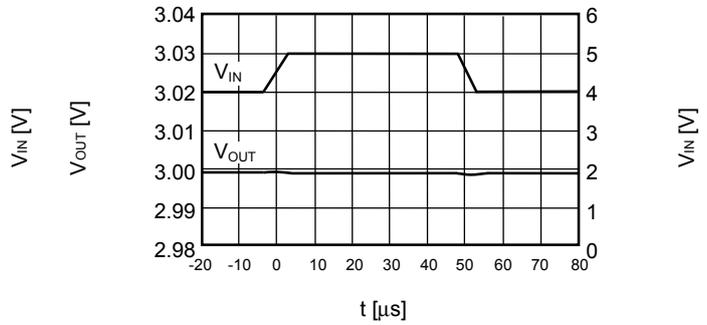
$I_{OUT} = 30\text{ mA}$ ,  $t_r = t_f = 5.0\ \mu\text{s}$ ,  $C_{OUT} = 2.2\ \mu\text{F}$ ,  $C_{IN} = 0\ \mu\text{F}$
