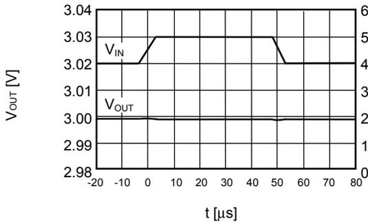
$I_{OUT} = 30\text{ mA}$ ,  $t_r = t_f = 5.0\ \mu\text{s}$ ,  $C_{OUT} = 1.0\ \mu\text{F}$ ,  $C_{IN} = 0\ \mu\text{F}$
