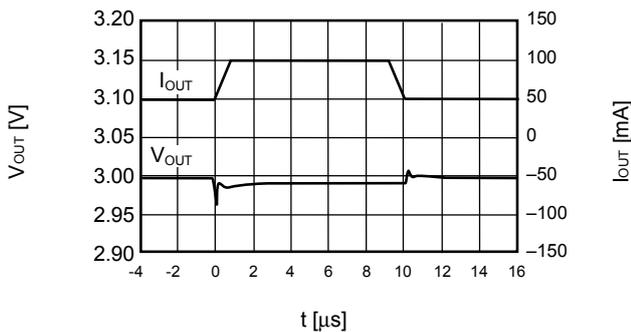
**(3) ON/OFF pin transient response characteristics**
