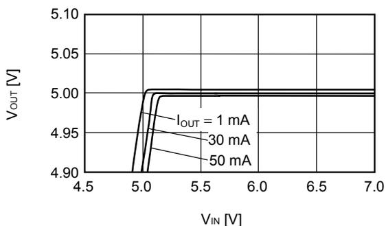
**(3) Dropout voltage vs. Output current**
