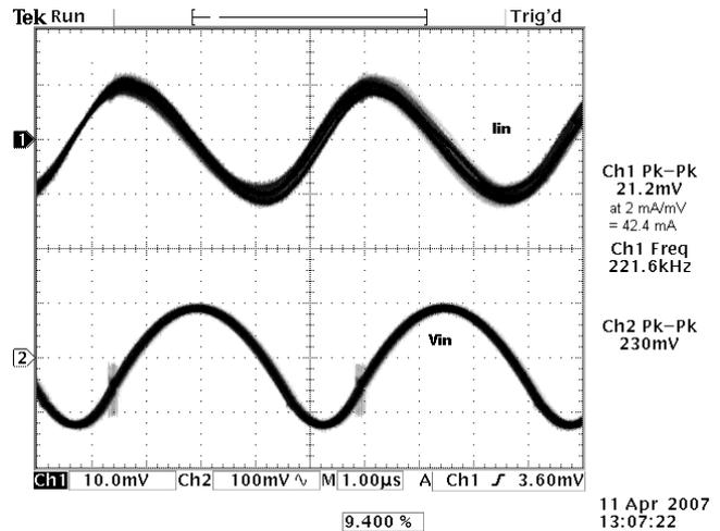
**Photo 2:** Input Ripple Voltage and Current
