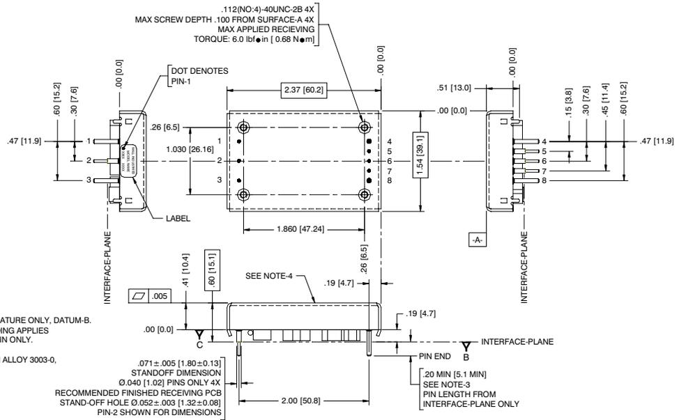
Mechanical Dimensions (Heatsink Option - "HS" suffix)
