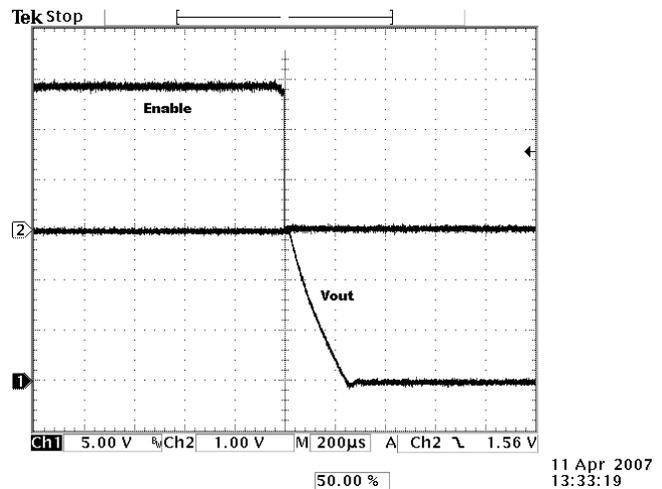
**Photo 6:** Turn Off by Enable at 24 V
