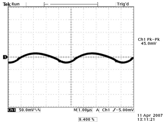
**Photo 8:** Output Ripple and Noise (20 MHz BW)
