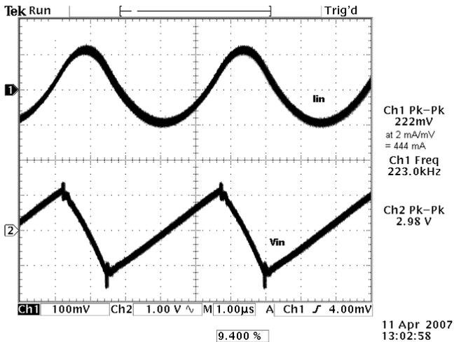
**Photo 1:** Input Ripple Voltage and Current
