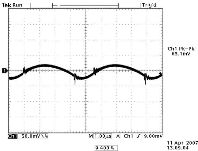
**Photo 7:** Output Ripple and Noise (20 MHz BW)
