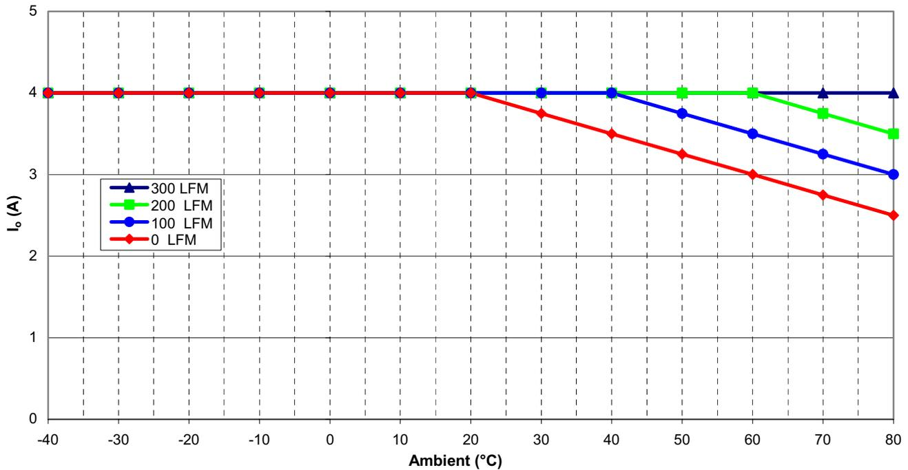
**Note 3:** When trimming output high,  $I_o$  vs. Ambient is derated by power. ie: from Graph 2, find the maximum current at the desired ambient and airflow, and multiply this current by the nominal voltage to get the maximum power. Divide this power by the desired trimmed high voltage to get the maximum current at that ambient. When trimming low, the maximum current stays the same as shown in Graph 2.
