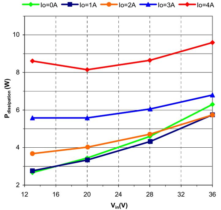
**Graph 5:** MPQ24S15-50C No Load Input Current and Power Dissipation vs. Input Voltage
