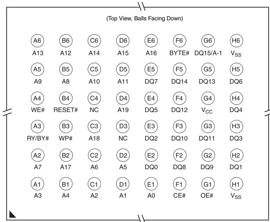
**Figure 3.3** 64-ball Fortified BGA
