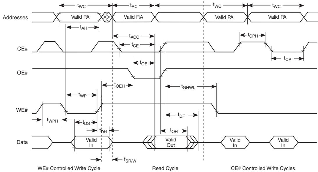
Figure 17.8 Data# Polling Timings (During Embedded Algorithms)
