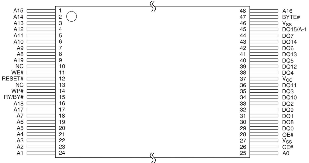
Figure 3.2 48-ball Fine-pitch BGA (VBK048)
