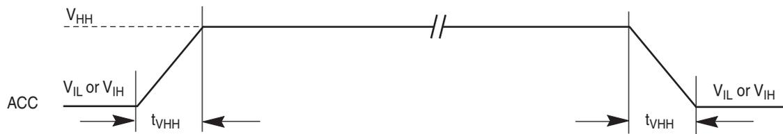
Figure 15.7 Chip/Sector Erase Operation Timings
