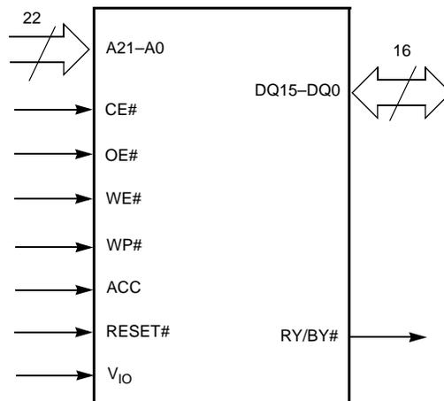
**Figure 5.4** S29GL032N Logic Symbol (Models 01, 02, V1, V2)
