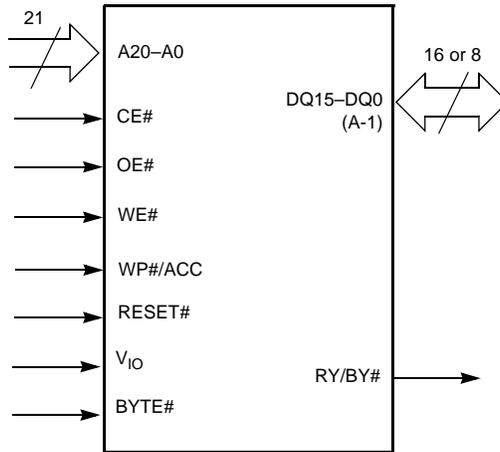
**Figure 5.5** S29GL032N Logic Symbol (Models 03, 04)
