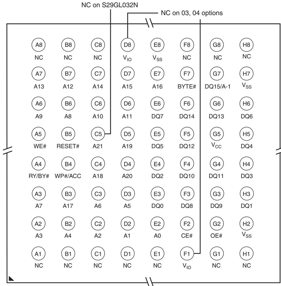
**Figure 3.4** 48-ball Fine-pitch BGA (VBK 048)
