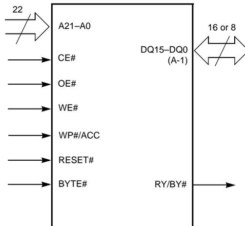
Figure 5.3 S29GL064N Logic Symbol (Models 06, 07, V6, V7)
