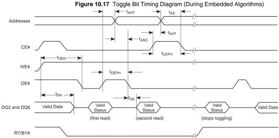
Note: 1. DQ6 will toggle at any read address while the device is busy. DQ2 will toggle if the address is within the actively erasing sector.
