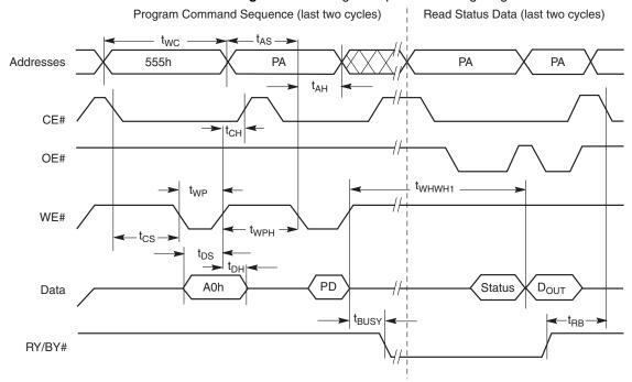
Figure 10.14 Program Operation Timing Diagram
