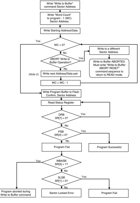
Figure 5.3 Write Buffer Programming Operation with Status Register
