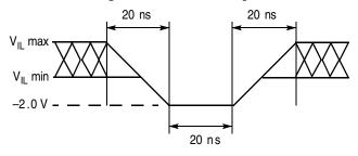
Figure 9.4 Maximum Positive Overshoot Waveform
