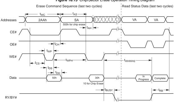
Figure 10.15 Chip/Sector Erase Operation Timing Diagram
