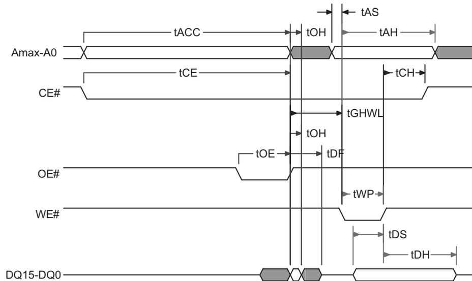
**Figure 10.13** Read to Write (CE# Toggle) Operation Timing Diagram
