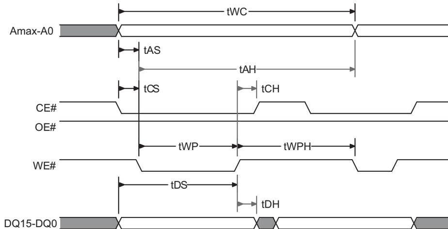
**Figure 10.9** Back to Back (CE#VIL) Write Operation Timing Diagram
