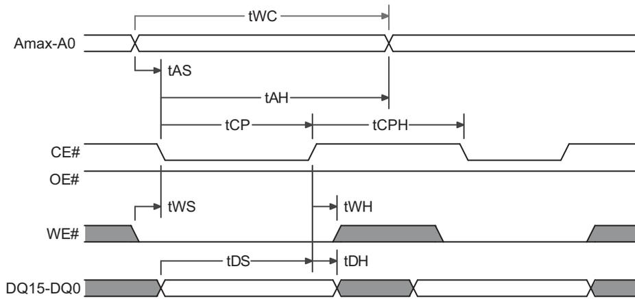
**Figure 10.20** (CE#) Write to Read Operation Timing Diagram
