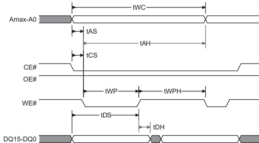
**Figure 10.10** Write to Read ( $t_{ACC}$ ) Operation Timing Diagram
