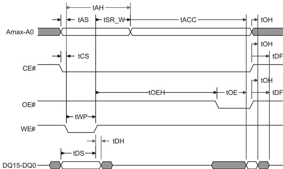
**Figure 10.11** Write to Read ( $t_{CE}$ ) Operation Timing Diagram
