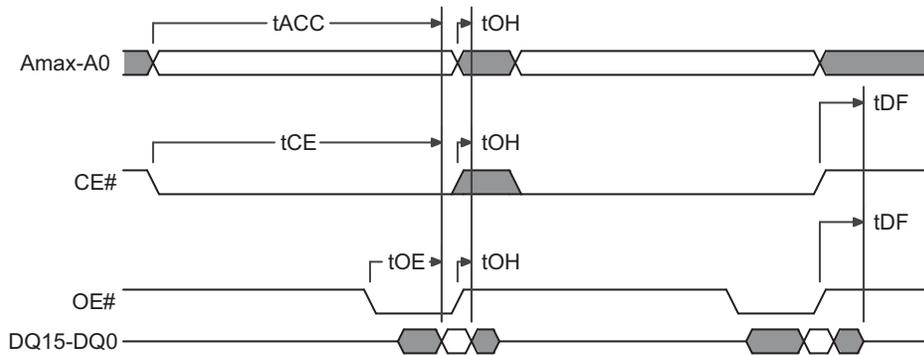
**Figure 10.6** Back to Back Read Operation ( $t_{RC}$ ) Timing Diagram
