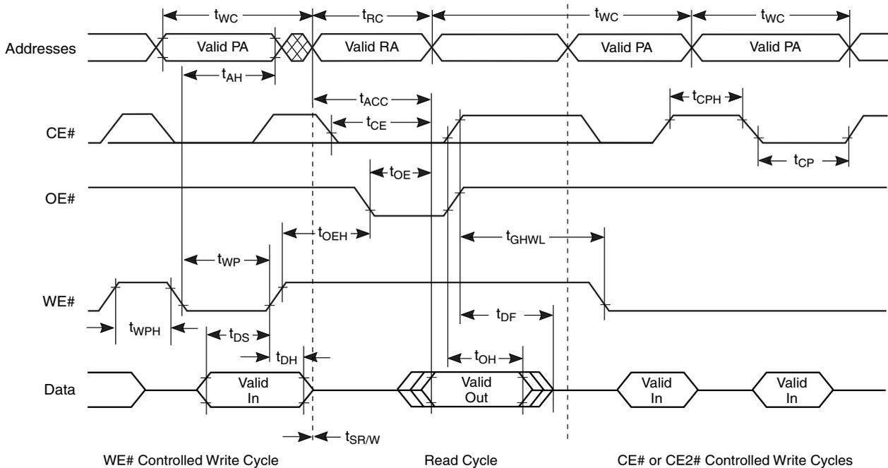
**Figure 17.9 Data# Polling Timings (During Embedded Algorithms)**
