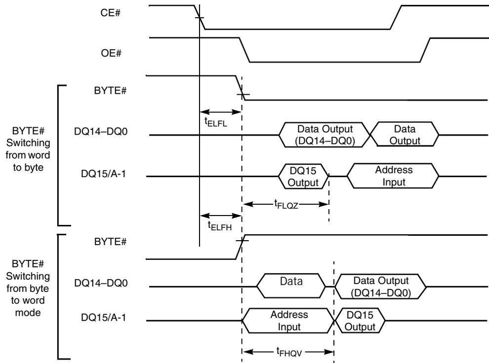
Figure 17.4 BYTE# Timings for Write Operations
