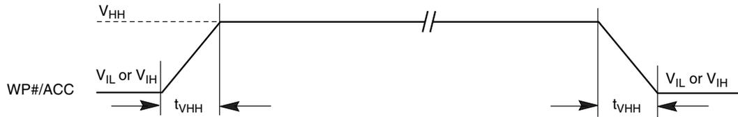
Figure 17.7 Chip/Sector Erase Operation Timings
