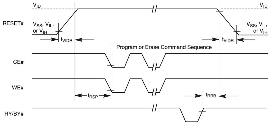
Figure 17.13 Sector/Sector Block Protect and Unprotect Timing Diagram
