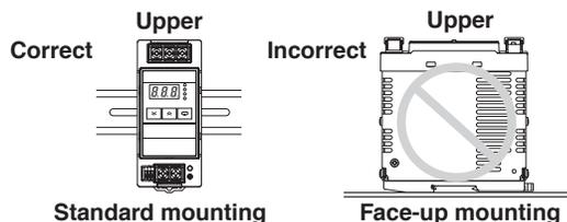
**Note:** Improper mounting will interfere with heat dissipation and may occasionally result in deterioration or damage of internal parts. It may also result in failure of the maintenance forecast monitor function. Use the standard mounting method only.
