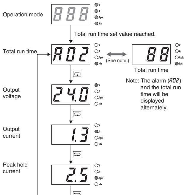
The accumulated value of the operating time of the Power Supply is displayed as the total run time. 0 (kh) will be displayed initially after purchase and then the display will advance in 1-kh steps as the operating time accumulates. When the total run time reaches the alarm set value, the alarm (R02) and the total run time will be displayed alternately and a transistor (total run time output terminal (kh)) will output the status externally.
