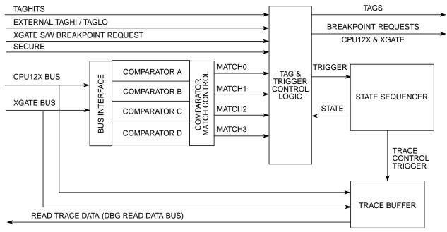
Figure 22-1. Debug Module Block Diagram
