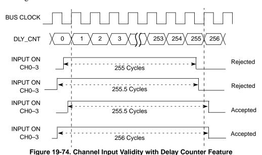
In Figure 19-74 a delay counter value of 256 bus cycles is considered.
