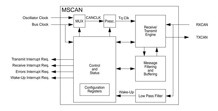
Figure 14-1. MSCAN Block Diagram
