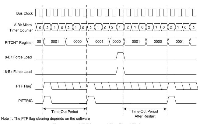
Figure 17-20. PIT Trigger and Flag Signal Timing
