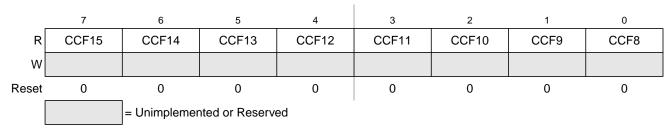
Figure 9-12. ATD Status Register 2 (ATDSTAT2)
