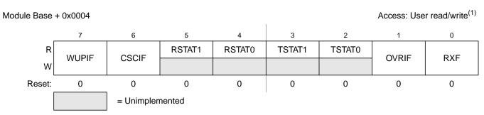
Figure 14-8. MSCAN Receiver Flag Register (CANRFLG)
