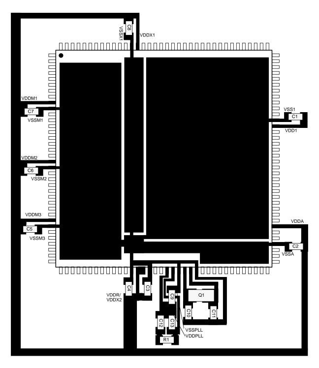
Figure C-1. LQFP144 Recommended PCB Layout
