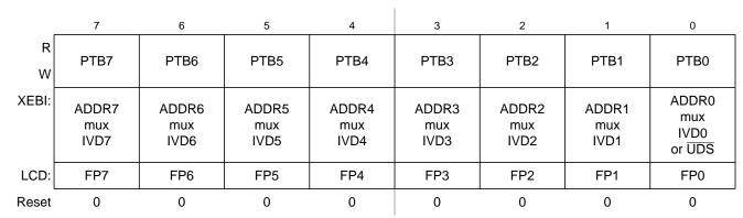
Figure 2-3. Port B I/O Register (PTB)
