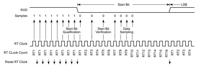
Figure 15-21. Receiver Data Sampling
