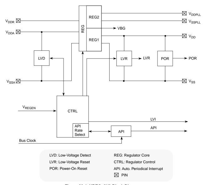
Figure 20-1. VREG\_3V3 Block Diagram
