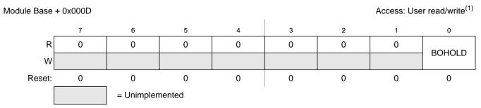
Figure 14-17. MSCAN Miscellaneous Register (CANMISC)
