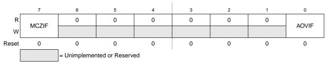
Figure 12-5. Stepper Stall Detector Flag Register (SSDFLG)
