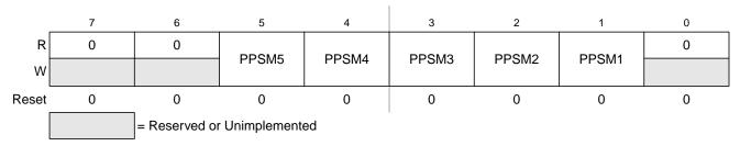
Figure 2-39. Port M Polarity Select Register (PPSM)
