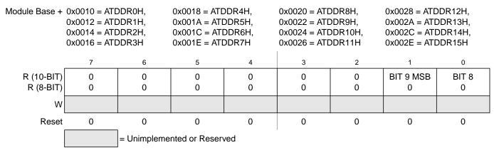
Figure 9-20. Right Justified, ATD Conversion Result Register x, High Byte (ATDDRxH)
