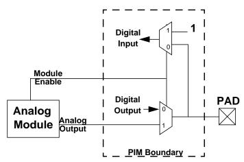
Figure 2-85. Digital Ports and Analog Module
