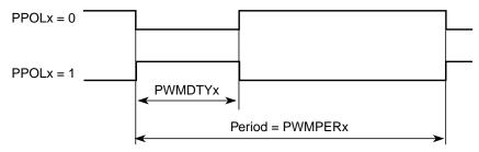
Figure 18-20. PWM Left Aligned Output Waveform
