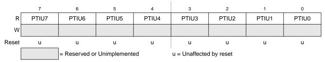
Figure 2-67. Port U Input Register (PTIU)
