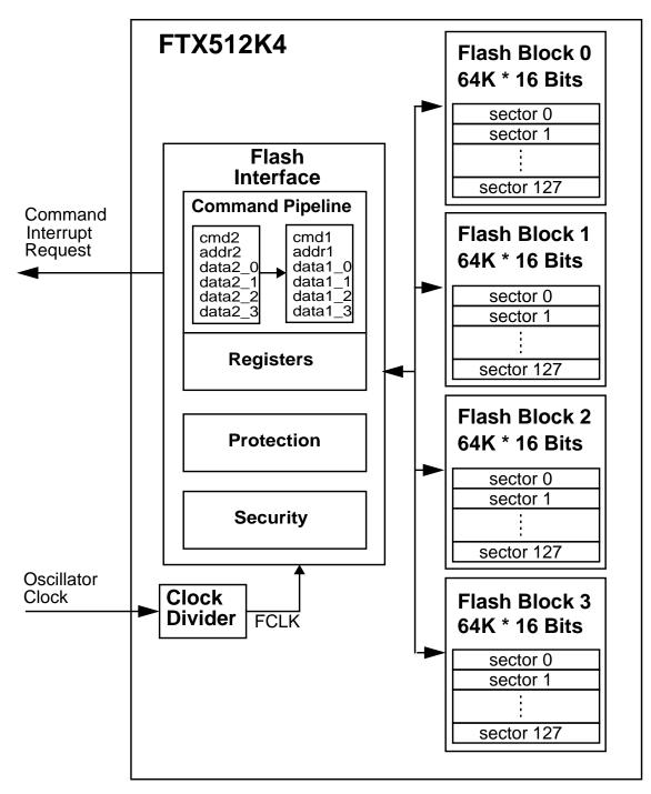
Figure 3-1. FTX512K4 Block Diagram
