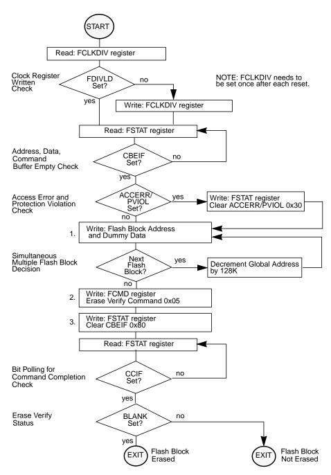
Figure 3-25. Example Erase Verify Command Flow
