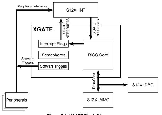
Figure 5-1. XGATE Block Diagram
