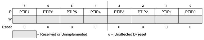
Figure 2-43. Port P I/O Register (PTP)
