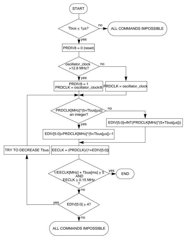
Figure 4-17. Determination Procedure for PRDIV8 and EDIV Bits
