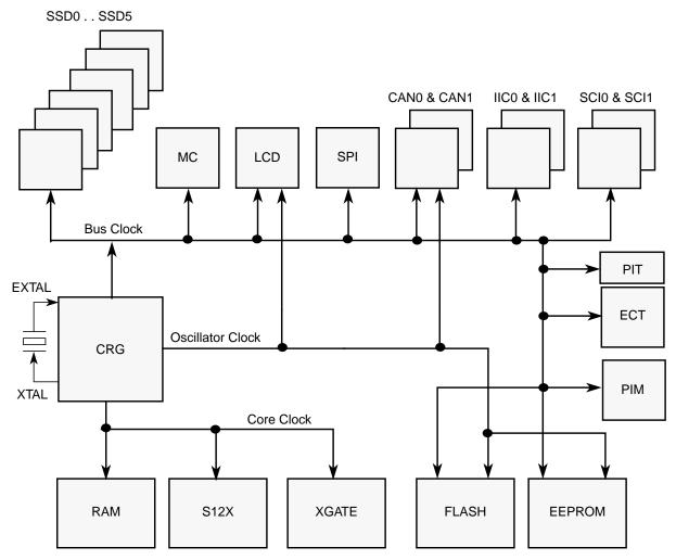
Figure 1-10. Clock Connections
