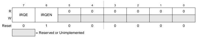
Figure 2-17. Port E Data Direction Register (DDRE)
