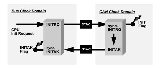
Figure 14-45. Initialization Request/Acknowledge Cycle
