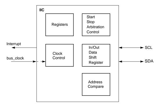
Figure 13-1. IIC Block Diagram
