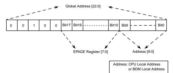
Figure 25-14. EPAGE Address Mapping
