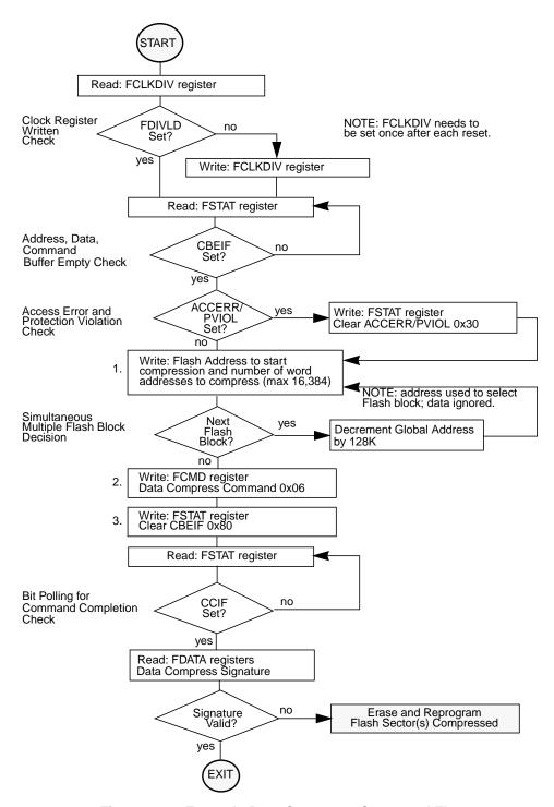
Figure 3-26. Example Data Compress Command Flow
