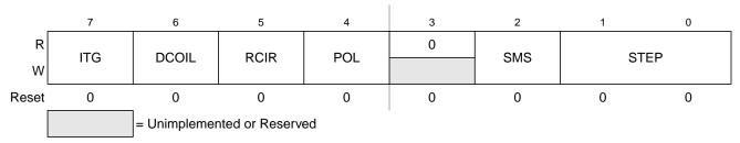
Figure 12-2. Return-to-Zero Control Register (RTZCTL)
