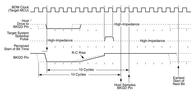
Figure 21-9. BDM Target-to-Host Serial Bit Timing (Logic 1)
