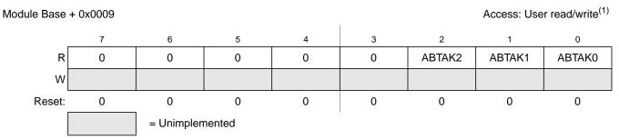
Figure 14-13. MSCAN Transmitter Message Abort Acknowledge Register (CANTAAK)
