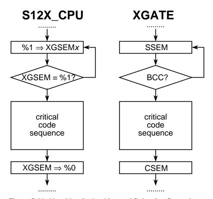
Figure 5-22. Algorithm for Locking and Releasing Semaphores
