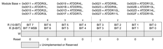
Figure 9-21. Right Justified, ATD Conversion Result Register x, Low Byte (ATDDRxL)
