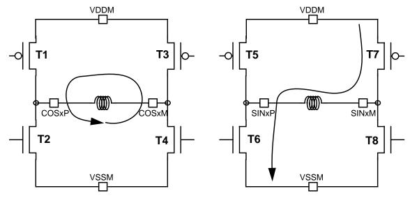
Figure 12-14. Current flow when STEP = 3, DCOIL = 1, ITG = 1
