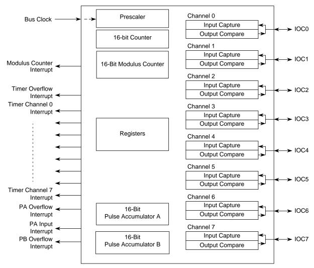
Figure 19-1. ECT Block Diagram
