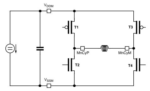
Figure 11-16. Output Transistor Assignment
