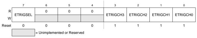
Figure 9-4. ATD Control Register 1 (ATDCTL1)
