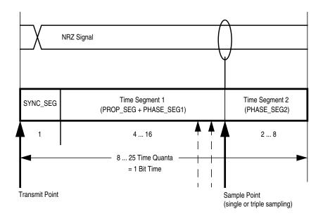
Figure 14-44. Segments within the Bit Time
