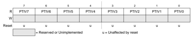
Figure 2-73. Port V Input Register (PTIV)
