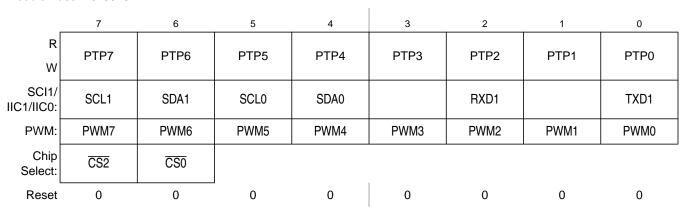
Figure 2-42. Port P I/O Register (PTP)
