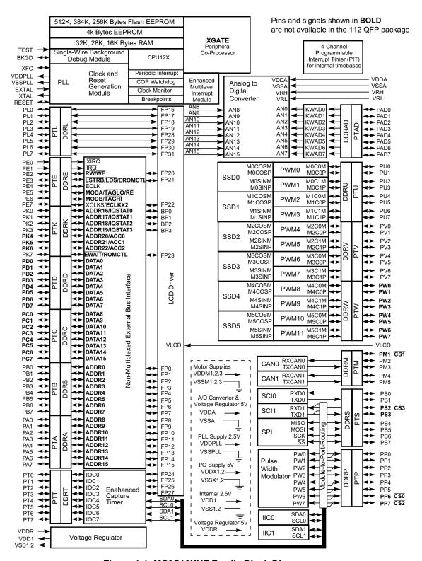
Figure 1-1. MC9S12XHZ Family Block Diagram
