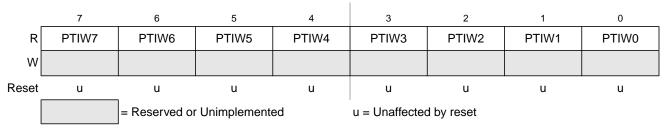
Figure 2-79. Port W Input Register (PTIW)
