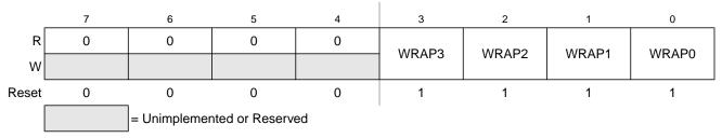
Figure 9-3. ATD Control Register 0 (ATDCTL0)
