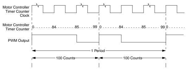
Figure 11-20. PWM Output: DITH = 1, MCAM[1:0] = 10, MCDC = 31, MCPER = 200, RECIRC = 0
