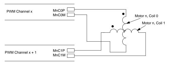
Figure 11-10. Typical Dual Full H-Bridge Mode Configuration
