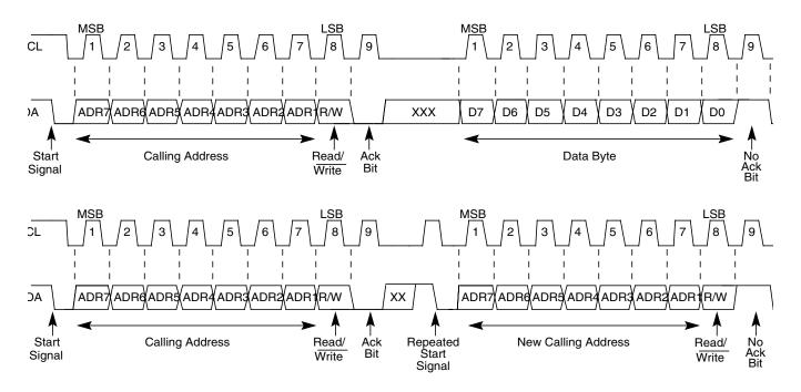
Figure 13-10. IIC-Bus Transmission Signals
