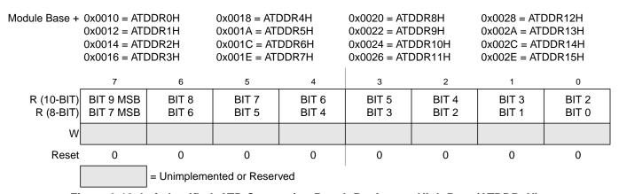
Figure 9-18. Left Justified, ATD Conversion Result Register x, High Byte (ATDDRxH)
