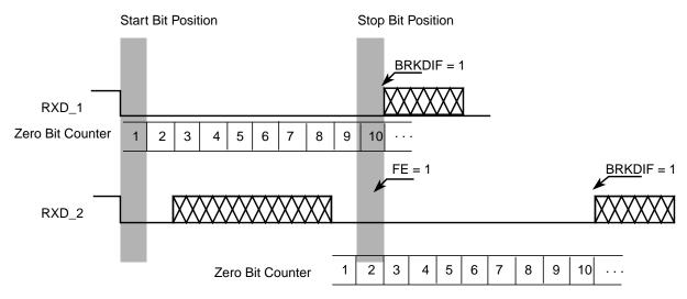
Figure 15-17. Break Detection if BRKDFE = 1 (M = 0)
