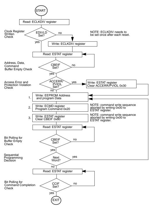
Figure 4-19. Example Program Command Flow
