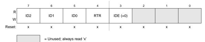
Figure 14-31. Identifier Register 1 — Standard Mapping
