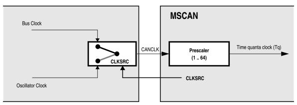
Figure 14-43. MSCAN Clocking Scheme
