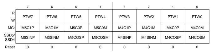
Figure 2-78. Port W I/O Register (PTW)
