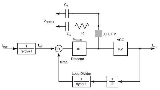
Figure A-3. Basic PLL Functional Diagram
