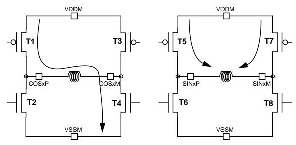
Figure 12-11. Current Flow when STEP = 0, DCOIL = 1, ITG = 0, RCIR = 0
