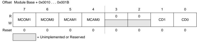
Figure 11-7. Motor Controller Control Register Channel 0... 11 (MCCC 0... MCCC11)
