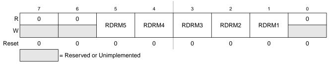
Figure 2-37. Port M Reduced Drive Register (RDRM)
