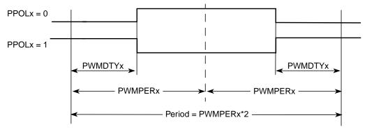
Figure 18-22. PWM Center Aligned Output Waveform
