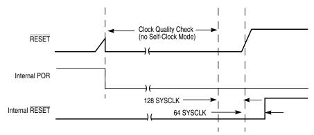
Figure 7-26. RESET Pin Tied to V<sub>DD</sub> (by a pull-up resistor)
