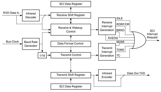
Figure 15-1. SCI Block Diagram
