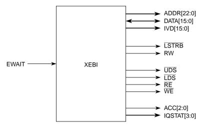
Figure 23-1. XEBI Block Diagram
