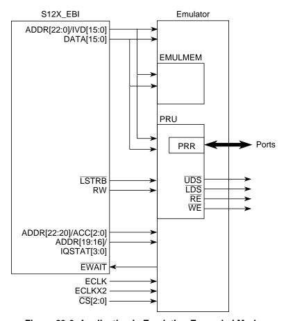
Figure 23-6. Application in Emulation Expanded Mode
