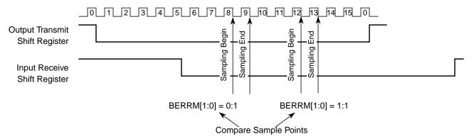
Figure 15-19. Timing Diagram Bit Error Detection
