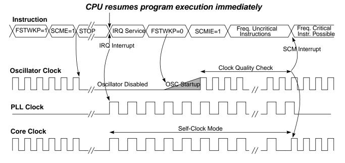
Figure 7-24. Fast Wake-up from Full Stop Mode: Example 2
