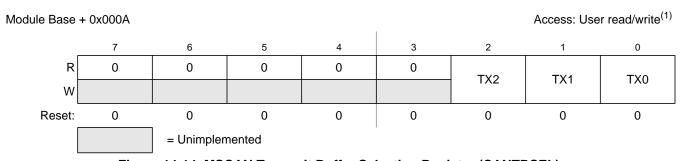
Figure 14-14. MSCAN Transmit Buffer Selection Register (CANTBSEL)
