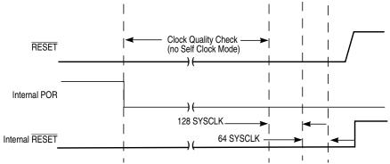
Figure 7-27. RESET Pin Held Low Externally
