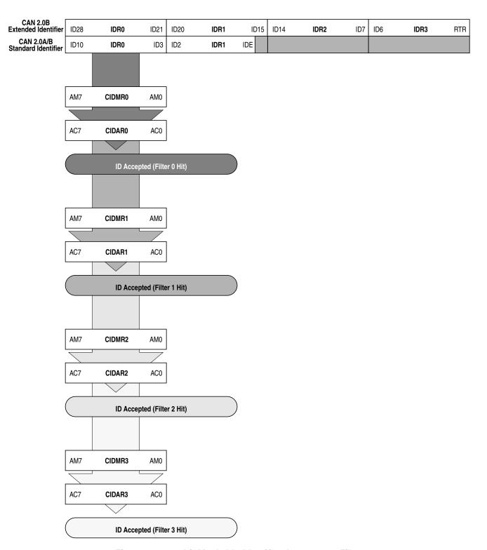
Figure 14-42. 8-bit Maskable Identifier Acceptance Filters
