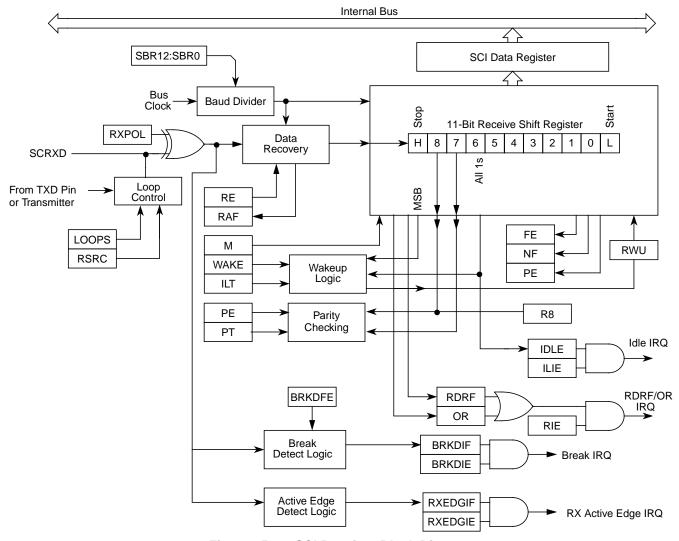
Figure 15-20. SCI Receiver Block Diagram
