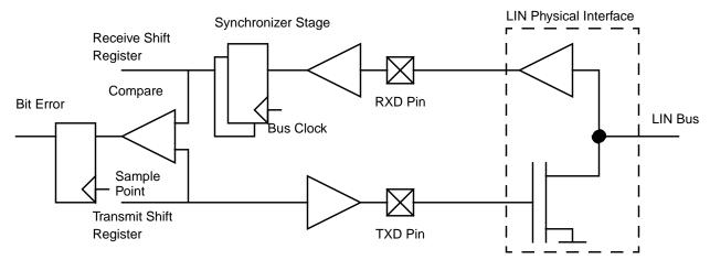
Figure 15-18. Collision Detect Principle
