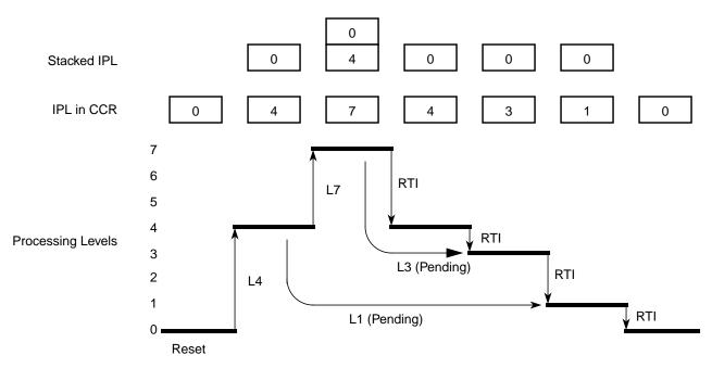
Figure 24-14. Interrupt Processing Example
