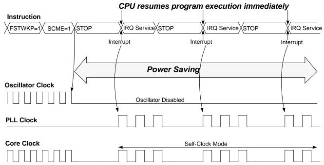
Figure 7-23. Fast Wake-up from Full Stop Mode: Example 1
