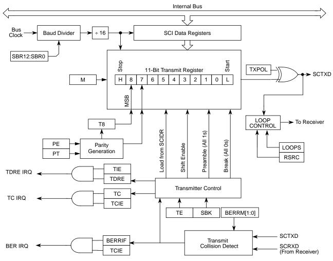
Figure 15-16. Transmitter Block Diagram
