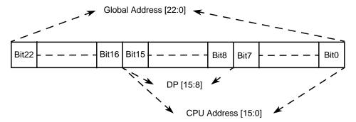
Figure 25-9. DIRECT Address Mapping
