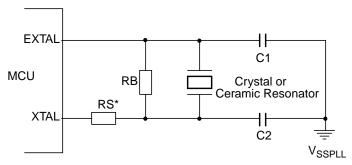
$<sup>^{\</sup>ast}$  R  $_{s}$  can be zero (shorted) when use with higher frequency crystals. Refer to manufacturer's data.
