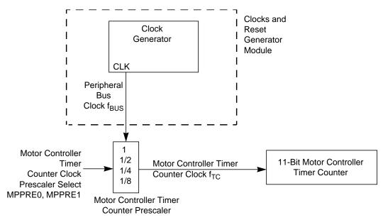
Figure 11-22. Motor Controller Counter Clock Selection
