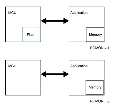
Figure 25-29. ROM in Normal Expanded Mode
