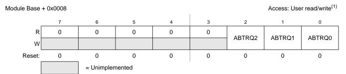
Figure 14-12. MSCAN Transmitter Message Abort Request Register (CANTARQ)
