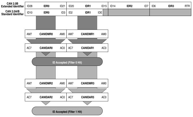
Figure 14-41. 16-bit Maskable Identifier Acceptance Filters
