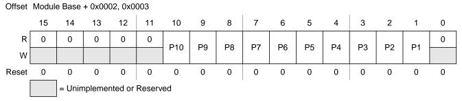
Figure 11-6. Motor Controller Period Register (MCPER) with DITH = 1
