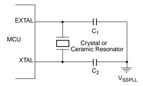
Figure 1-7. Loop Controlled Pierce Oscillator Connections (PE7 = 0)
