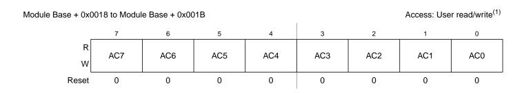
Figure 14-21. MSCAN Identifier Acceptance Registers (Second Bank) — CANIDAR4-CANIDAR7
