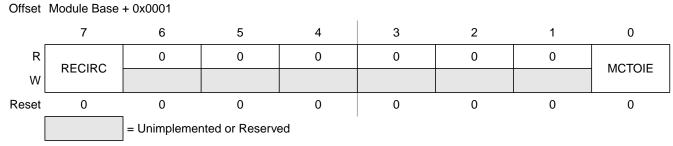
Figure 11-4. Motor Controller Control Register 1 (MCCTL1)
