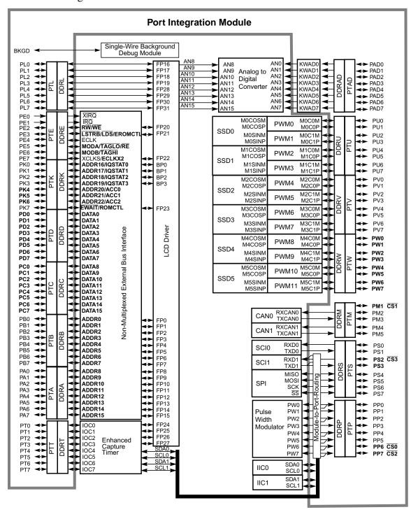
Figure 2-1. S12XHZPIM Block Diagram
