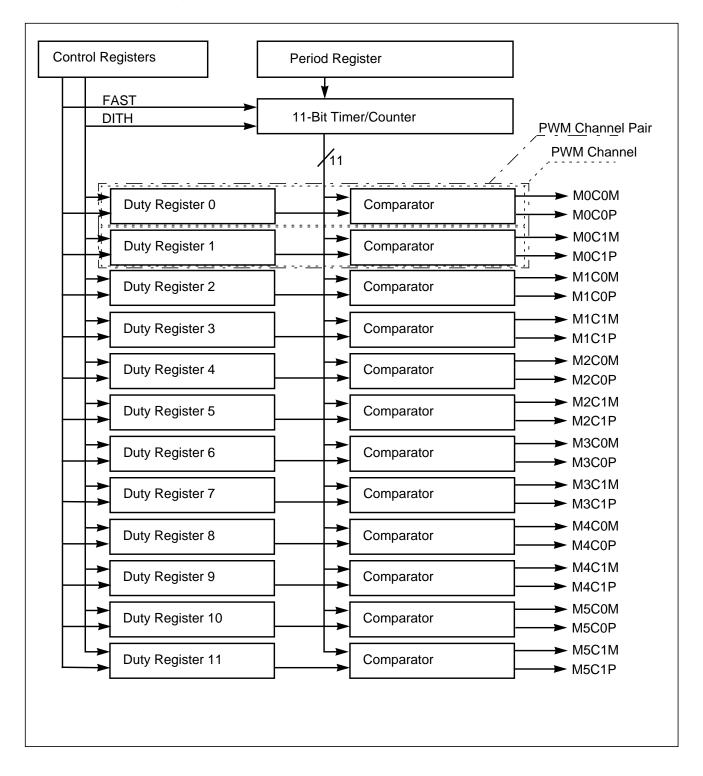
Figure 11-1. MC10B12C Block Diagram
