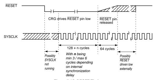
Figure 7-25. RESET Timing
