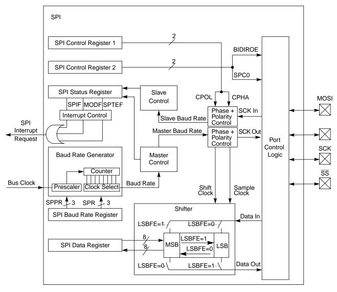
Figure 16-1. SPI Block Diagram
