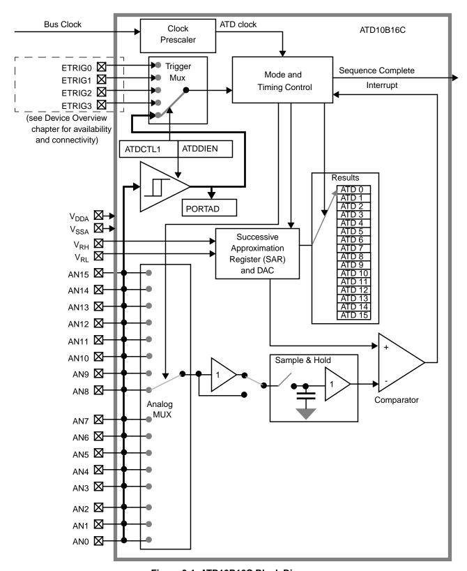
Figure 9-1. ATD10B16C Block Diagram
