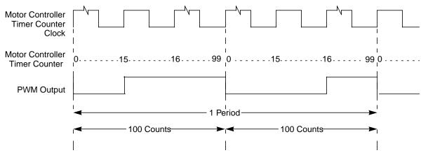
Figure 11-18. PWM Output: DITH = 1, MCAM[1:0] = 01, MCDC = 31, MCPER = 200, RECIRC = 0
