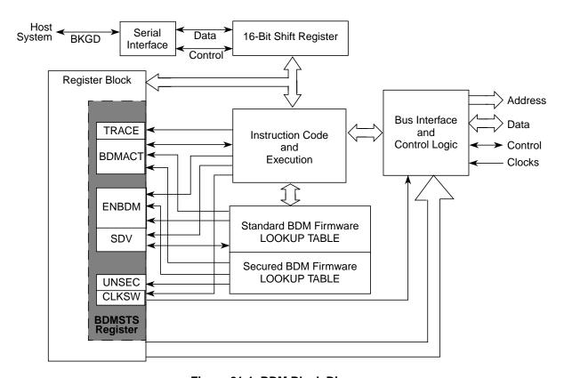
Figure 21-1. BDM Block Diagram
