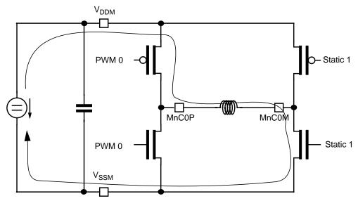
Figure 11-14. PWM Active Phase, RECIRC = 1, S = 0
