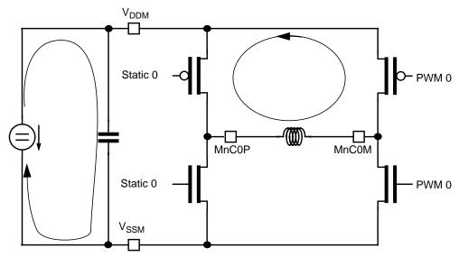
Figure 11-13. PWM Passive Phase, RECIRC = 0, S = 0
