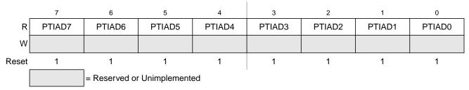
Figure 2-20. Port AD Input Register (PTIAD)
