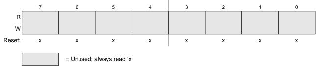
Figure 14-33. Identifier Register 3 — Standard Mapping
