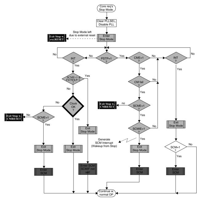
Figure 7-22. Stop Mode Entry/Exit Sequence
