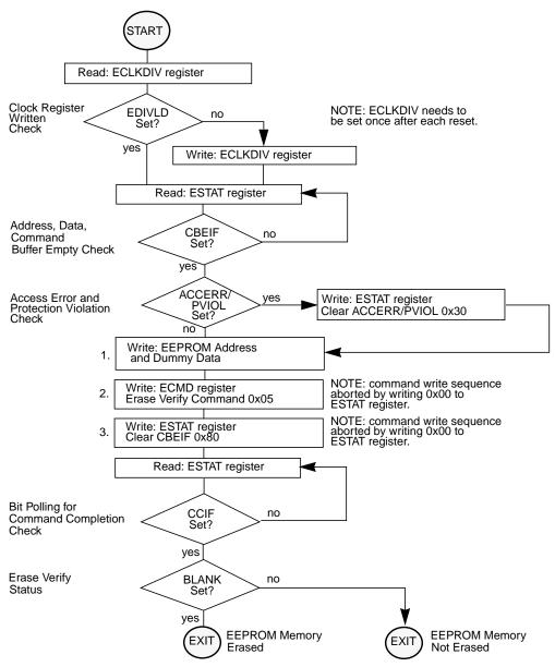
Figure 4-18. Example Erase Verify Command Flow
