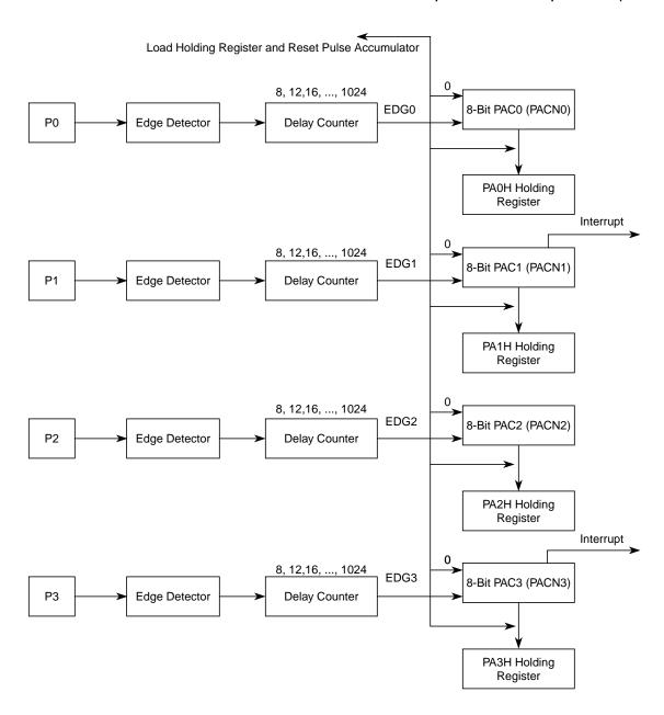
Figure 19-71. 8-Bit Pulse Accumulators Block Diagram
