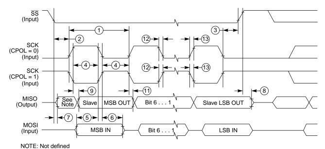
Figure A-9. SPI Slave Timing (CPHA = 1)
