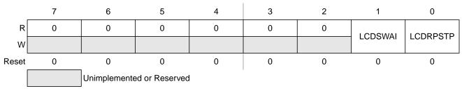
Figure 10-3. LCD Control Register 1 (LCDCR1)
