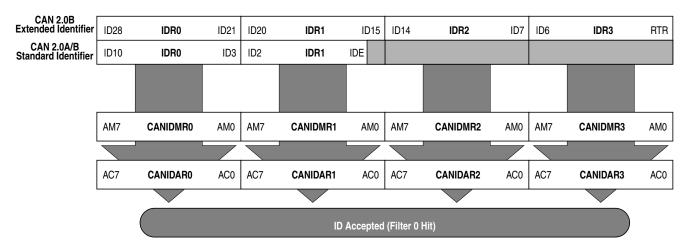
Figure 14-40. 32-bit Maskable Identifier Acceptance Filter
