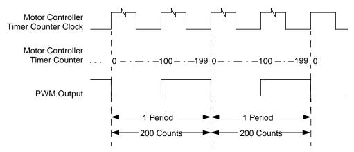
Figure 11-17. PWM Output: DITH = 0, MCAM[1:0] = 01, MCDC = 100, MCPER = 200, RECIRC = 0
