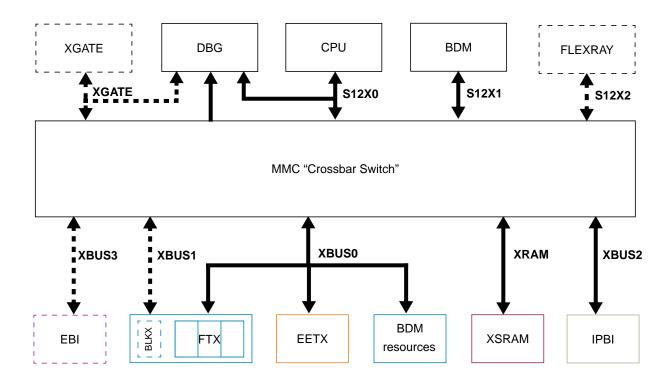
Figure 25-26. MMC Block Diagram
