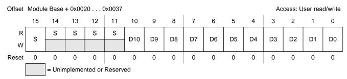
Figure 11-8. Motor Controller Duty Cycle Register x (MCDCx) with FAST = 0
