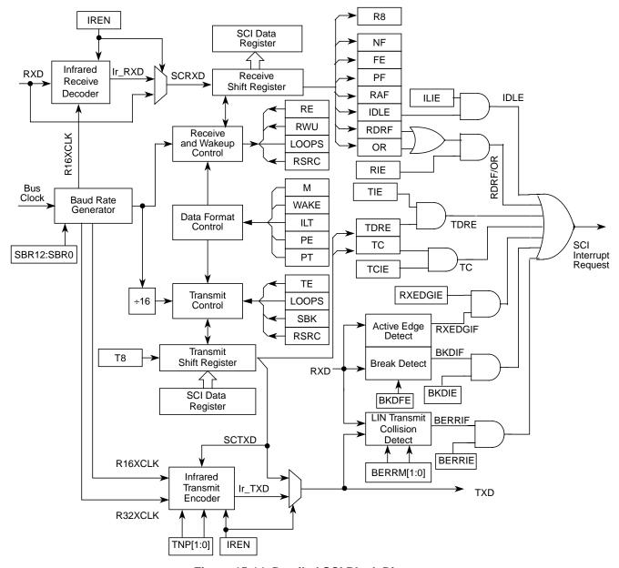
Figure 15-14. Detailed SCI Block Diagram
