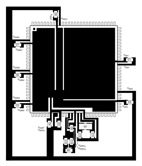
Figure C-2. LQFP112 Recommended PCB Layout
