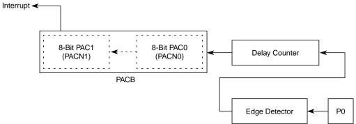
Figure 19-72. 16-Bit Pulse Accumulators Block Diagram
