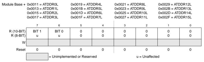
Figure 9-19. Left Justified, ATD Conversion Result Register x, Low Byte (ATDDRxL)
