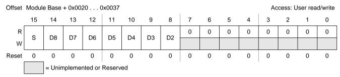
Figure 11-9. Motor Controller Duty Cycle Register x (MCDCx) with FAST = 1
