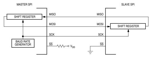
Figure 16-10. Master/Slave Transfer Block Diagram
