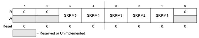
Figure 2-41. Port M Slew Rate Register (SRRM)
