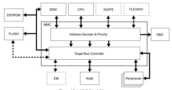
Figure 25-1. MMC Block Diagram
