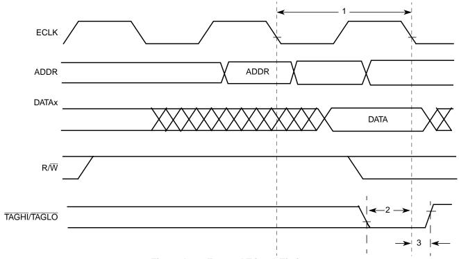
Figure A-16. External Trigger Timing
