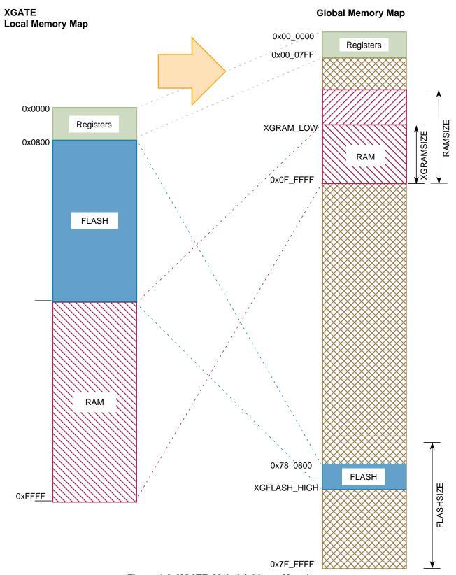
Figure 1-3. XGATE Global Address Mapping
