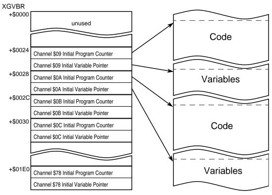
Figure 5-20. XGATE Vector Block
