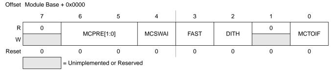
Figure 11-3. Motor Controller Control Register 0 (MCCTL0)
