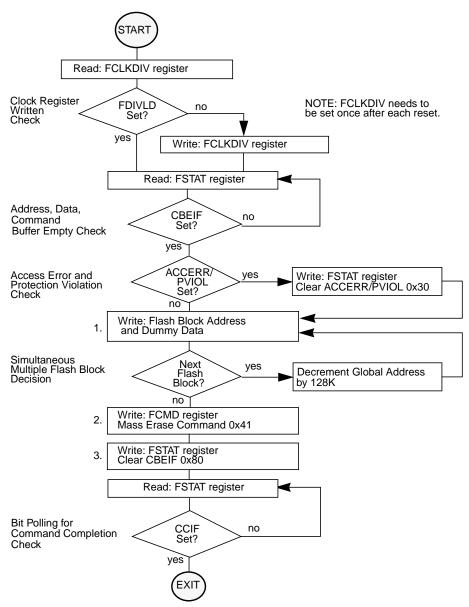
Figure 3-30. Example Mass Erase Command Flow
