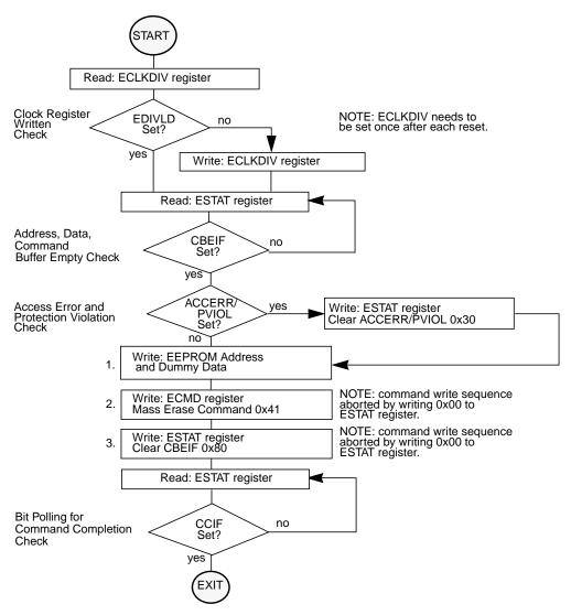
Figure 4-21. Example Mass Erase Command Flow
