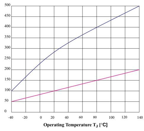
Figure A-2. Typical Endurance vs Temperature
