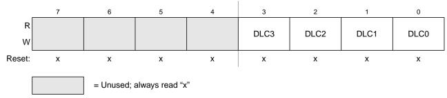
Figure 14-35. Data Length Register (DLR) — Extended Identifier Mapping
