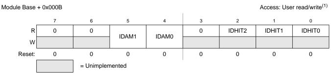
Figure 14-15. MSCAN Identifier Acceptance Control Register (CANIDAC)
