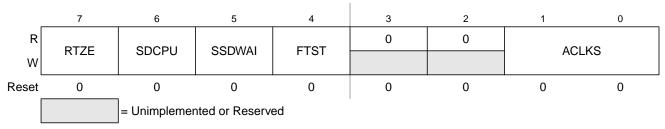
Figure 12-4. Stepper Stall Detector Control Register (SSDCTL)
