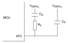
Figure 1-6. PLL Loop Filter Connections
