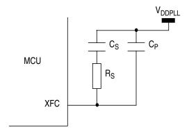
Figure 7-2. PLL Loop Filter Connections
