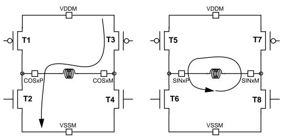
Figure 12-13. Current flow when STEP = 2, DCOIL = 1, ITG = 1
