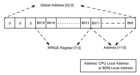
Figure 25-12. RPAGE Address Mapping
