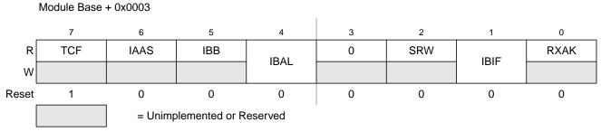
Figure 13-7. IIC Bus Status Register (IBSR)
