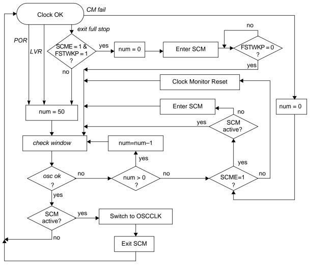
Figure 7-20. Sequence for Clock Quality Check
