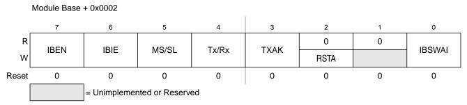
Figure 13-6. IIC Bus Control Register (IBCR)
