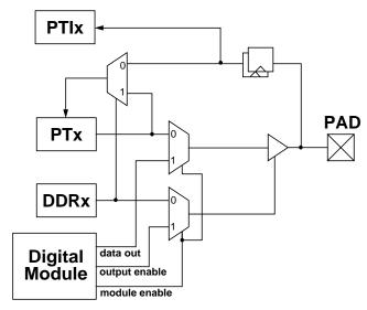
Figure 2-84. Illustration of I/O Pin Functionality
