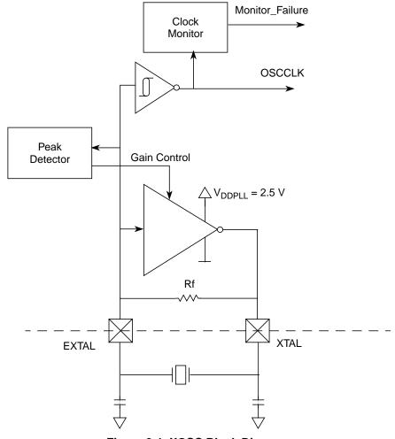
Figure 8-1. XOSC Block Diagram
