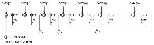
Figure 3-27. 16-Bit MISR Diagram
