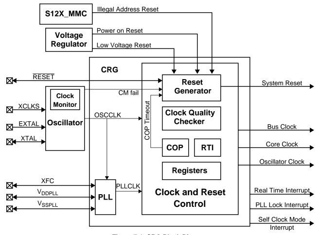
Figure 7-1. CRG Block Diagram
