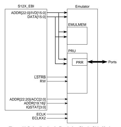
Figure 23-5. Application in Emulation Single-Chip Mode
