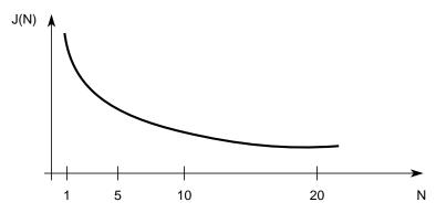
Figure A-5. Maximum Bus Clock Jitter Approximation
