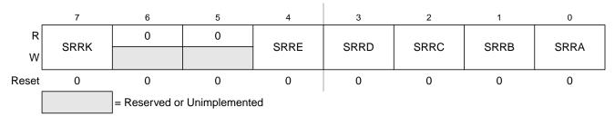
Figure 2-18. Slew Rate Control Register (SRCR)
