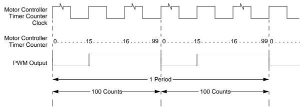
Figure 11-19. PWM Output: DITH = 1, MCAM[1:0] = 01, MCDC = 30, MCPER = 200, RECIRC = 0
