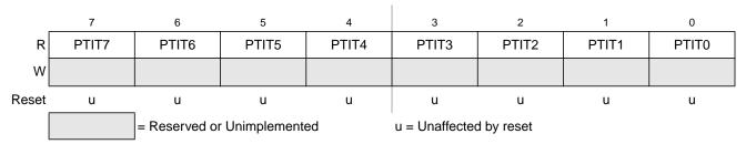
Figure 2-59. Port T Input Register (PTIT)
