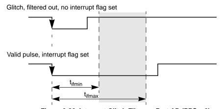
Figure 2-86. Interrupt Glitch Filter on Port AD (PPS = 0)
