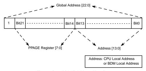
Figure 25-16. PPAGE Address Mapping
