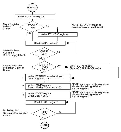
Figure 4-23. Example Sector Modify Command Flow
