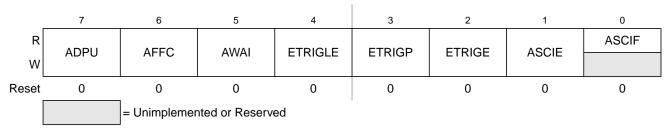
Figure 9-5. ATD Control Register 2 (ATDCTL2)
