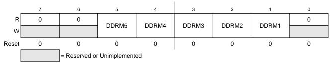
Figure 2-36. Port M Data Direction Register (DDRM)
