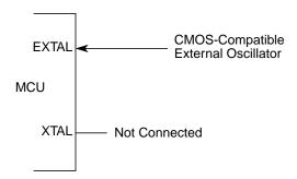
Figure 1-9. External Clock Connections (PE7 = 1)
