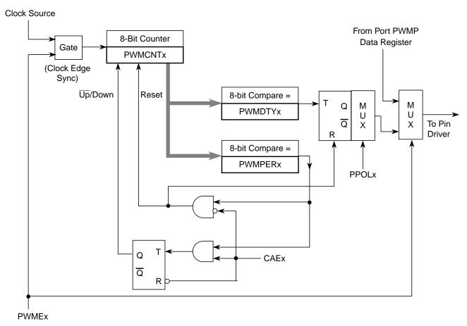
Figure 18-19. PWM Timer Channel Block Diagram
