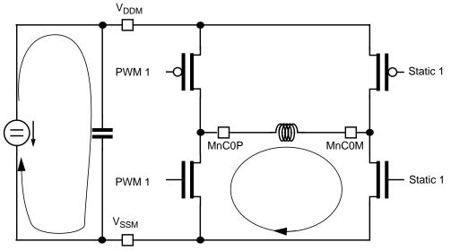
Figure 11-15. PWM Passive Phase, RECIRC = 1, S = 0
