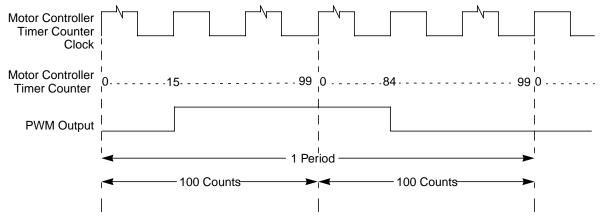
Figure 11-21. PWM Output: DITH = 1, MCAM[1:0] = 11, MCDC = 31, MCPER = 200, RECIRC = 0
