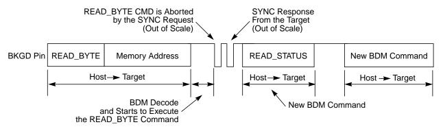
Figure 21-13. ACK Abort Procedure at the Command Level
