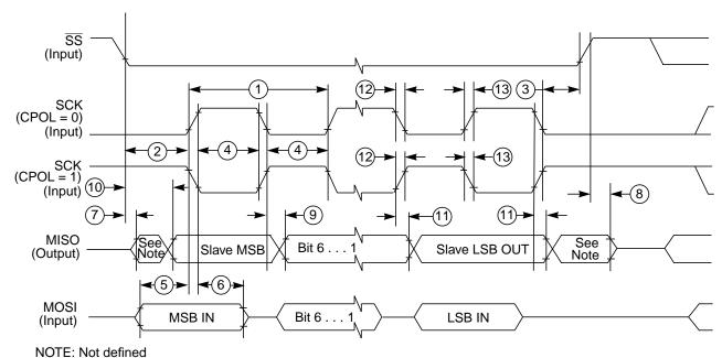
Figure A-8. SPI Slave Timing (CPHA = 0)
