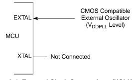
Figure 8-4. External Clock Connections (XCLKS = 1)
