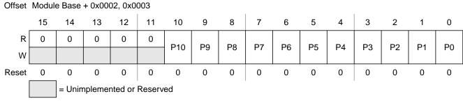
Figure 11-5. Motor Controller Period Register (MCPER) with DITH = 0
