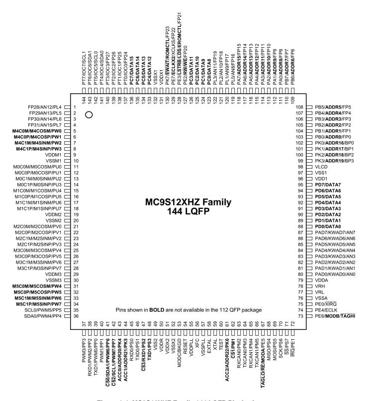
Figure 1-4. MC9S12XHZ Family 144 LQFP Pin Assignment
