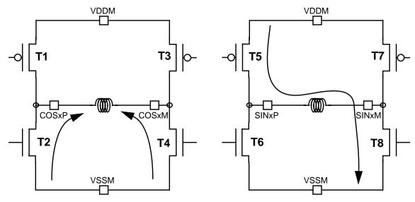
Figure 12-12. Current Flow when STEP = 1, DCOIL = 1, ITG = 0, RCIR = 1
