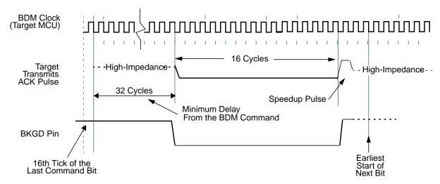
Figure 21-11. Target Acknowledge Pulse (ACK)
