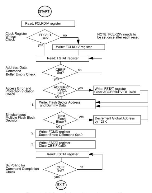
Figure 3-29. Example Sector Erase Command Flow
