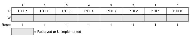
Figure 2-28. Port L Input Register (PTIL)
