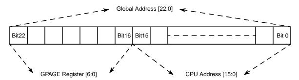
Figure 25-7. GPAGE Address Mapping
