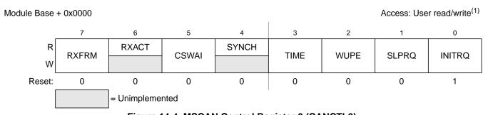
Figure 14-4. MSCAN Control Register 0 (CANCTL0)
