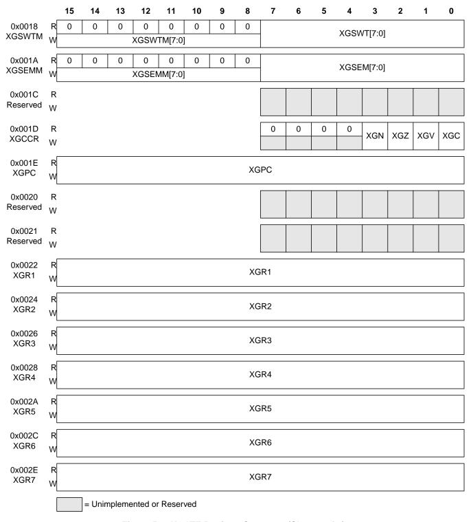
Figure 5-2. XGATE Register Summary (Sheet 3 of 3)
