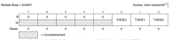
Figure 14-11. MSCAN Transmitter Interrupt Enable Register (CANTIER)
