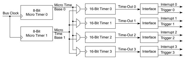
Figure 17-1. PIT Block Diagram
