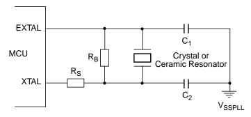
Figure 1-8. Full Swing Pierce Oscillator Connections (PE7 = 1)
