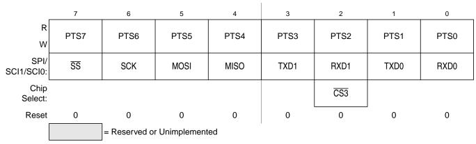
Figure 2-50. Port S I/O Register (PTS)
