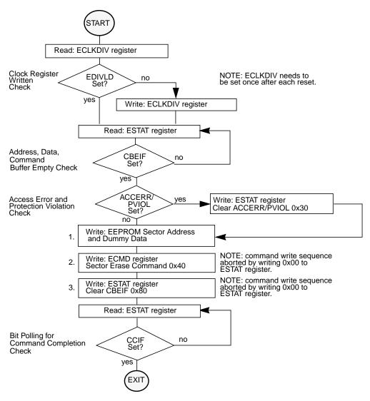
Figure 4-20. Example Sector Erase Command Flow
