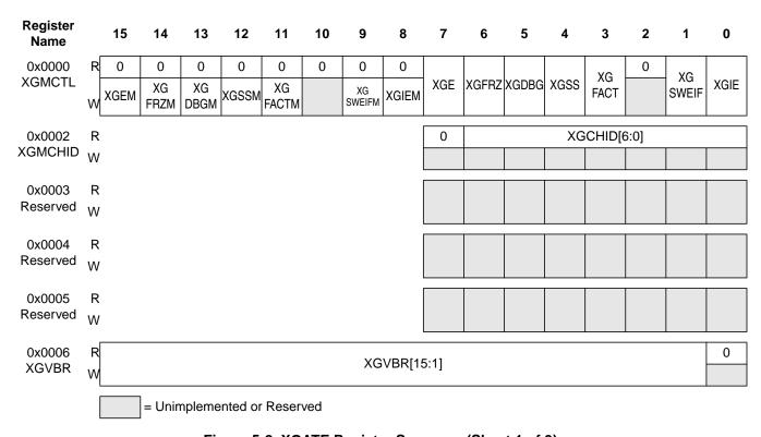
Figure 5-2. XGATE Register Summary (Sheet 1 of 3)
