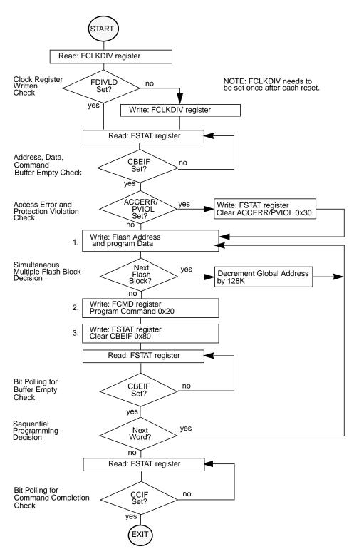
Figure 3-28. Example Program Command Flow
