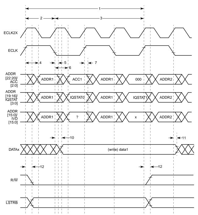
Figure A-15. Example 2b: Emulation Expanded Mode — Write with 1 Stretch Cycle
