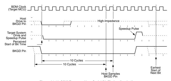
Figure 21-10. BDM Target-to-Host Serial Bit Timing (Logic 0)
