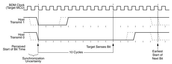
Figure 21-8. BDM Host-to-Target Serial Bit Timing
