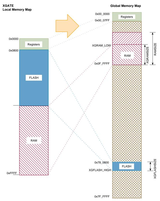
Figure 25-24. XGATE Global Address Mapping
