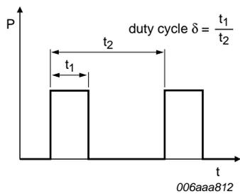
Fig 17. Duty cycle definition
