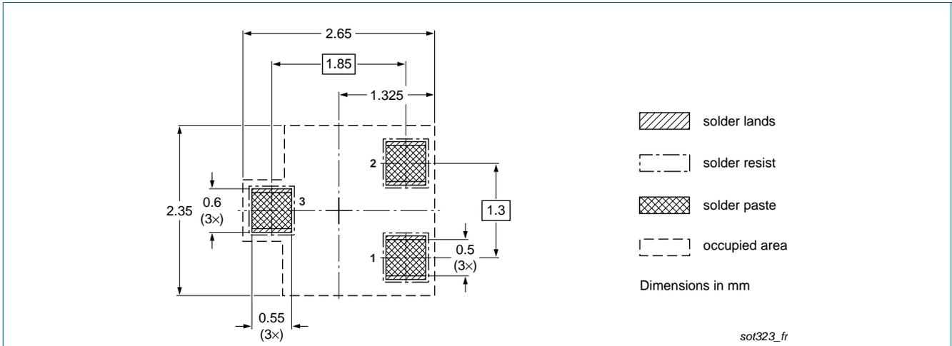
Fig 19. Reflow soldering footprint for SOT323 (SC-70)
