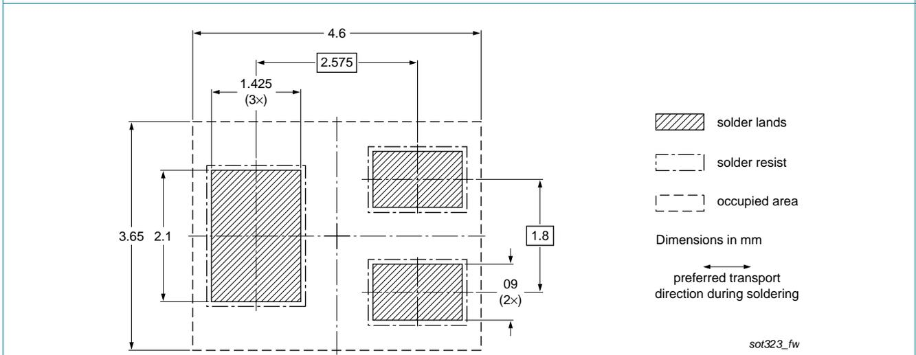
Fig 20. Wave soldering footprint for SOT323 (SC-70)
