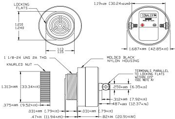
NOTE B: MOUNTING- REMOVE BLACK PLASTIC NUT AND INSERT THREADED FRONT THROUGH 1.25' HOLE PUNCHED IN PANEL, IF ORIENTATION IS NEEDED, NOTE LOCKING FLATS ON DRAWING. SCREW NUT BACK ON. DO NOT OVERTIGHTEN.
