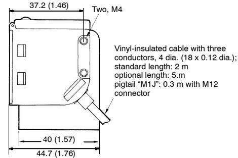
Note: The output switch, mode switch, and distance setting knob can be accessed by removing the cover.
