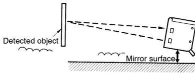
Mount the Sensor so that it is not aligned with the direction of movement of the detected object, as shown below.
