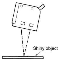
If stable operation is not possible near a mirror surface, mount the Sensor at an angle as shown below, and separate the Sensor as far as possible from the mirror surface.
