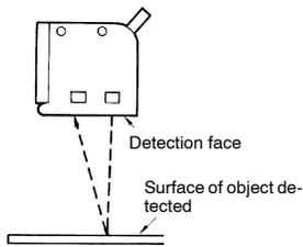
If detecting a shiny object, mount the Sensor so that the detection face is at an angle of between 5° and 10° of the surface of the object being detected. Check to be sure that there is no interference from the background (see below).
